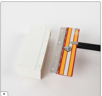
Align the hinge of the compartment door with the compartment inner, applying a little glue between the four lugs
