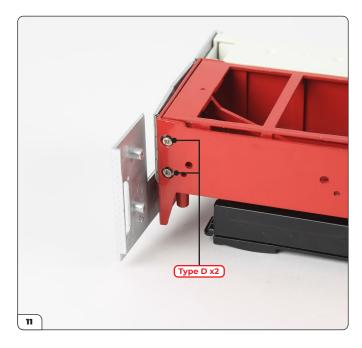
With the door in the closed position, secure it in place using  $2\,\mathrm{x}$  TYPE D screws, driving them in from the outside of the frame.
