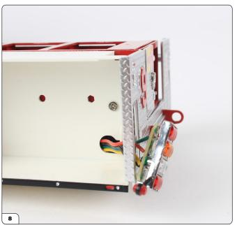
Pull the cable through as far as it will go until the PCB is held against the rear panel. Push this left side of the rear panel fully into place on the box frame, but leave the right side detached (see next image).
