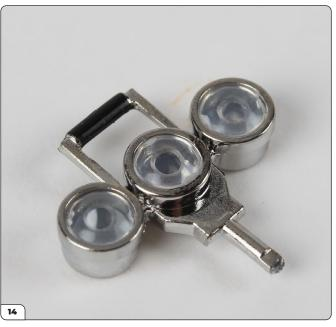
Apply a little PVA glue around the circular recesses before dropping the lenses into place.
