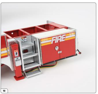
Gently push the storage compartment in place until the doors are flush to the compartment inner frame.
