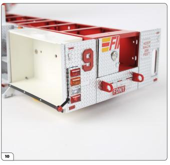
Pull the cable of the PCB tight amd push the light cluster fully into place so they sit flush on the rear panel.
