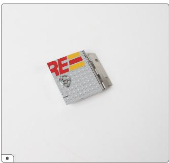
Turn the door the right way up and fix the handle in place in the D-shaped hole. Prepare to fix the door to the box frame shell.
