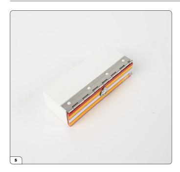
Glue the hinge over the lugs as shown, checking that the door closes correctly.
