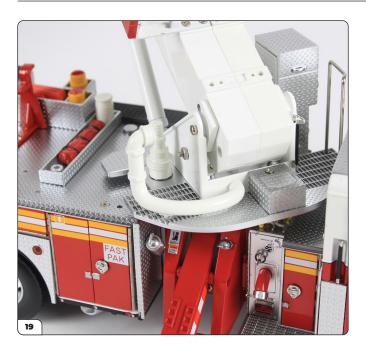
Push the water pipe into the fixing points in the orientation shown.
