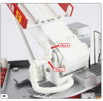
Push pipe c into the end of the water pipe; then add pipe b so that it faces in the same direction as the boom. **Do not glue** pipe b to pipe c as they must be free to move.
