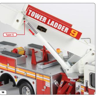
Slide the remaining piston from stage 47 into the piston tube. Fix the free end of the piston to the piston bracket with another Type G screw.
