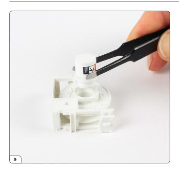
Align the flat notch on the reel motor with the notch in the reel. Push the cap through the bracket and into the reel.
