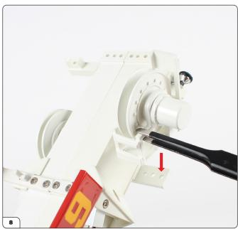
Align the pins on the bottom of the reel bracket with the reel support that was attached in the previous stage.
