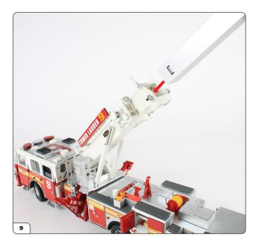
With the ladder guides facing up, slide the free end of the lower midsection into the bed section.
