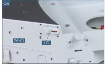
Identify the fixing point for the port navigation light housing on the bridge deck and check the fit. Apply a little superglue on the pegs of part **H3** and fix in place.
