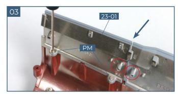
Fix hull section **23-01** in place with the screws. Don't worry if there is a gap between **23-01** and the forward section of the hull (indicated by the arrow). Identify the raised screw sockets (circled) where connector **23-02** will fit (see next step).
