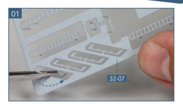
Take the metal frame **32-07** and remove all the parts: you can grip them with tweezers and twist them or use a side cutter to clip them from the frame. Use a fine file to remove any rough edges.
