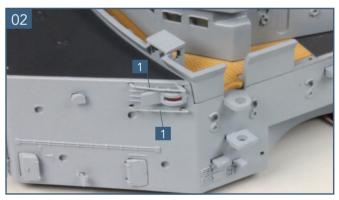
The first two metal parts are fitted above and below the port navigation light. Note the angle of the fixing bars at each end – the sharper angle goes at the rear.
