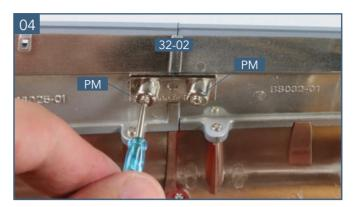
Fix part 32-02 in place with two PM screws.
