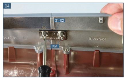
Fix the connector **31-02** in place with two **PM** screws.
