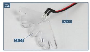
Fit the LED on the end of the **29-08** into the recess in the windows **29-05**.
