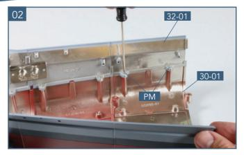
Fix part 32-01 to part 30-01 with two PM screws.
