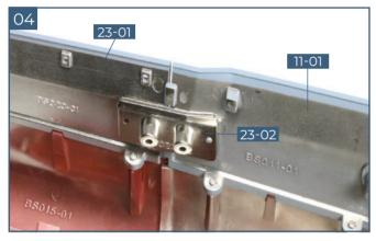
Fit the connector **23-02** on the raised screw sockets of the hull sections **23-01** and **11-01**.
