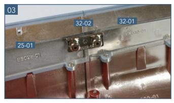
Fit the connector piece **32-02** in place across the join between parts **25-01** and **32-01** so that the raised screw holes fit into the sockets in part **32-02**.
