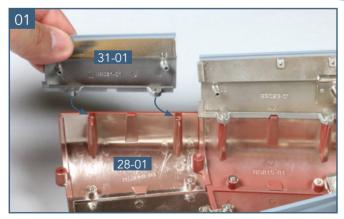
Place the hull assembly on your worksurface. Position the upper port hull section 31-01 on the structure so that the two tabs fit over the screw sockets in part 28-01, as indicated by the arrows.
