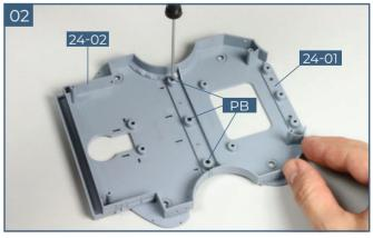
Turn the deck over and identify the three sockets along the overlap. Fix the parts together with three PB screws.
