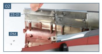
To fix the hull section in place you will need two **PM** 2 x 4 mm silver screws.
