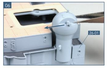
Check the fit of the rangefinder tower on the port side of the bridge deck **26-01**. Note that the rangefinder arms should point forwards. When you are happy with the position, glue in place.
