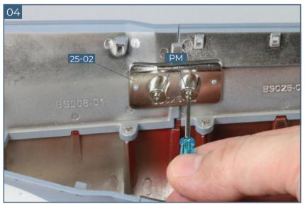
Fix the hull connector **25-02** in place with two **PM** screws.
