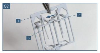
Fit the second part 3 in place through the opening in part 2, and glue the loop in place on the horizontal peg of part 1 with a little superglue.
