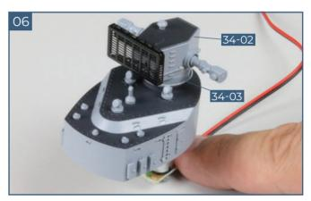
Check the fit of the radar unit **34-02** to the base of the radar unit **34-03** and check that the screw fitted earlier (see page 7 step 2) is fully tightened. Glue the radar unit in place.
