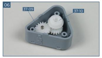
Fit cog **37-10** on the first shaft **37-11** so that its teeth engage with the outer ring of teeth on cog **37-09**.
