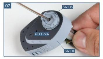
Attach the base of the radar unit 34-03 to the roof of the control centre using a **PB** (1.7 x 4 mm) screw.
