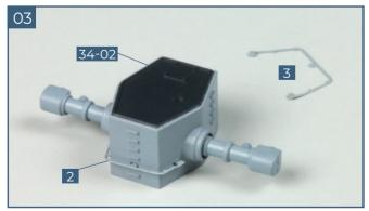
Cut parts 2 and 3 from the metal frame 34-13. Use a little glue to fix part 2 to the back of the radar unit 34-02, so that the three pins fit into the holes.
