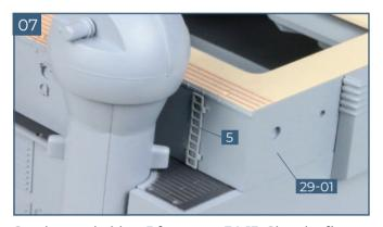
Cut the two ladders **5** from part **34-13**. Glue the first ladder **5** to the back port side of the superstructure (part **29-01**, behind the rangefinder).
