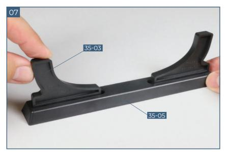
Next, fit the pegs on the other bracket **35-03** into the corresponding holes in the base **35-05**, as shown.
