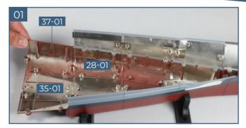
Take the hull assembly from stage 35. Fit the pegs on the lower port hull section **37-01** into the raised sockets in the hull sections **28-01** and **35-01**.
