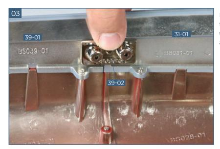
Fit the connecting piece **39-02** over the raised screw sockets on either side of the join between parts **39-01** and **31-01**.
