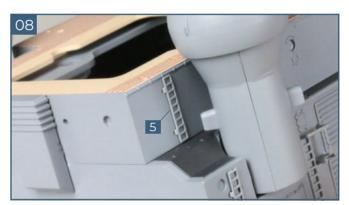
Glue the second ladder **5** to the starboard side of the superstructure, behind the rangefinder.
