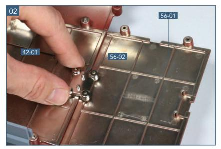
Fit the connector **56-02** over the four raised screw sockets on keel sections **42-01** and **56-01**.
