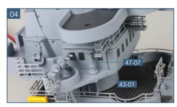
Glue the second compass **47-07** in place on the starboard side of the admiral's bridge **43-01**. As in the previous step, make sure it is facing the right way.
