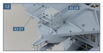
In the same way, glue the second platform **45-04** in place on the underside of the admiral's bridge deck **43-01**.
