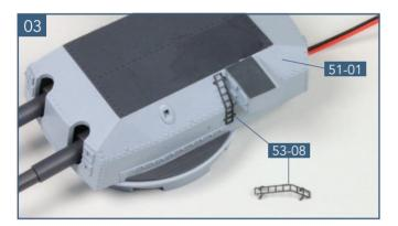
Take the first ladder **53-08** and fit the four pegs into the holes in the port side of the turret housing **51-01**. When you are happy with the fit, apply a little superglue to the pegs and fix in place.
