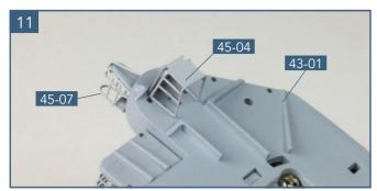
Turn the admiral's bridge deck assembly **43-01** upside down. Identify the fixing point for the first platform **45-04**. The open side should face towards the centre of the model. Fix in place with a little
