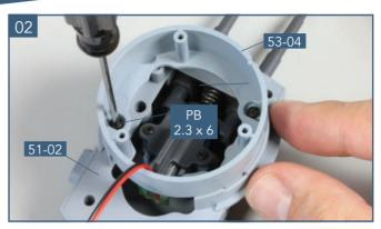
Fix the turret base **53-04** to part **51-02** with two 2.3 x 6mm **PB** screws.
