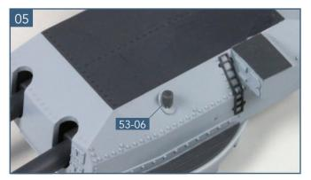
Cut the periscopes **53-06** from the frame. Fix the first one in place on the port side of the turret hood using a little superglue.
