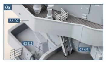
The ladder assembly from step 4 leads up from the searchlight deck **40-03** to the foretop gallery **38-02**. Identify the fixing point and glue the base of the ladder in place to the decking.
