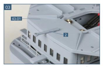
Identify the fixing point for antenna outrigger **2** and glue in place at the lower edge of the front of the admiral's bridge deck **43-01**, as shown.
