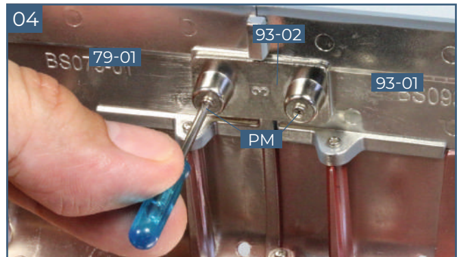
Fix the connector in place with two PM screws, as shown.
