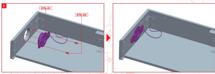
Insert the speaker 076-01 from Stage 76 into the pedestal assembled in Stage 79, and fix it with the two screws 076-05 that also came in Stage 76
