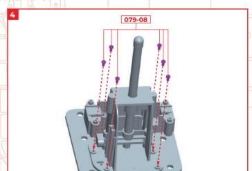
Fix the lifting device frame 079-03 in places with 6 x screws 079-08.
