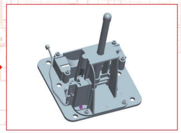
Fix the limit switch frame 069-02 with 1 x screw 079-08.
