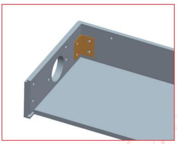
Align the metal fitting 071-02 that came with Stage 71 with the pedestal frames 069-04 and 079-05.
