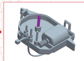
Insert the longer shaft of the camshaft 082-05 from under the gearbox 082-01.
