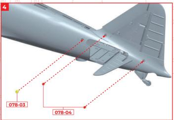
Fix one part of the left rear panel 075-01 with 1 x screw 078-03 and fix the right rear panel 078-01 with 2 x screws 078-04.
