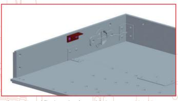
Align the metal fitting 084-03 with the pedestal frame parts 079-05 and 084-01, and fix them in place with  $2 \times 100$  screws 084-05.
