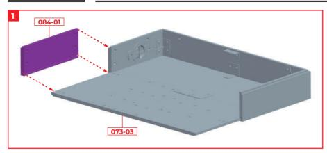
Fit the groove on the outer frame 084-01 into the pedestal plate 073-03 assembled in Stage 81.
