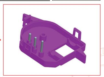
Insert three shafts 082-03 into the gearbox 082-01. Push firmly as the holes are quite narrow.
