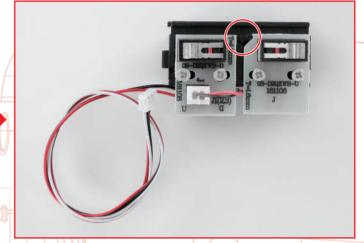
Fix the limit switch in place with 4 x 083-08 screws. Note that there is a little room to move the screw holes left and right. Check that the cut corner of the limit switch is aligned with the triangular protrusion on the board before tighteneing the screws to ensure correct alignment.
