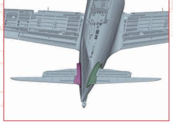
Insert the fairing (left) 074-04 that came with Stage 74 onto the elevator (left). Insert the fairing (right) 077-02 that came with Stage 77 onto the elevator (right). Insert the fairing all the way to the base and then push it forward so that it fits into the recess in the rear external panel.
