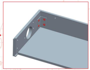
Fix the metal fitting in place with 4 x screws 071-07 that came with Stage 71.
