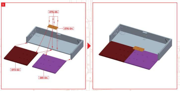
Align the pedestal plates 073-02 and 081-04 with the pedestal assembled in Stage 80, and the metal fitting 076-04 from Stage 76. Fix in place using 4 x screws 076-05.
