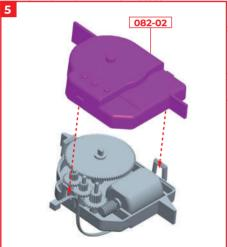
Cover the gearbox 082-01 with the gearbox lid 082-02 and fit the claws.
