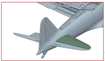
Apply superglue to the 5 pins on the underside of the right horizontal tail wing 080-02 and glue it to the underside of the right tail wing frame, then attach the right horizontal tail wing (topside) 080-01 from above.
