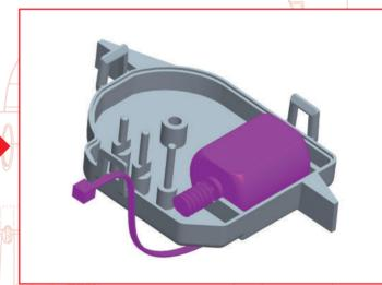
Feed the wire from motor 082-04 through the hole in gearbox 082-01 and fit the motor with the wire facing down.
