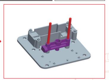
Insert the slider 079-01 onto the lifting device base 071-05 that came with Stage 71. Insert two shafts 079-02 through the slider into the lifting device base.
