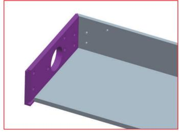
Fit the grooves on the pedestal frame 079-05 into the pedestal plates 072-03 and 069-04 of the pedestal assembled in Stage 72.
