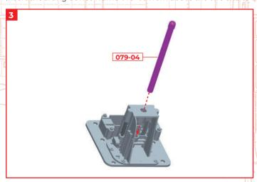
Insert the support bar 079-04 through the hole at the top of the lifting device frame 079-03 into the slider 079-01.
