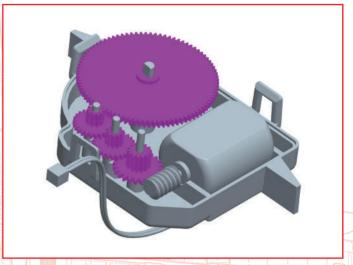
Insert gear 082-08 and 2 x gears 082-07 onto the three shafts 082-03 inserted in 1, in order, starting from the side closest to the motor. Make sure that the small gear faces upward. Finally, fit the gear 082-06 onto the camshaft 082-05 inserted in step 3 with the small gear facing down.
