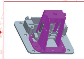
Insert the lifting device frame 079-03 from above the two shafts 079-02.
