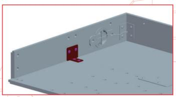
Align the metal fitting 084-02 with the pedestal frame parts 079-05 and 084-01, and fix in place with 4 x screws 084-05.
