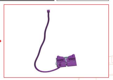
Fit the limit switch 083-03 into the frame 083-01, aligning the cut corners of the board of the limit switch 083-03 with the triangular protrusions on the frame 083-01.
