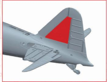
Fit the vertical stabiliser 075-03 that came with Stage 75 into place as shown.
