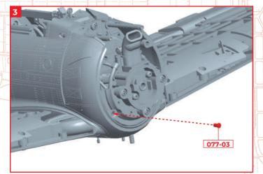
Fix the right front panel 077-01 with the screw 077-03 that came with Stage 77.
