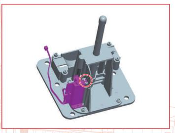
Slide the limit switch frame 069-02 assembled in Stage 69 into the groove on the lifting device frame 079-03 and fit it.
