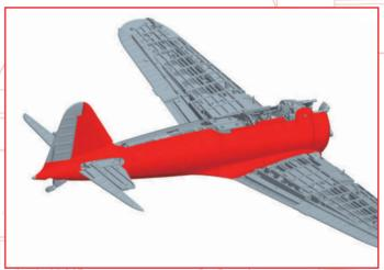
Fit the right external panel assembled in 1 from the right side of the fuselage. Insert the horizontal stabilizer into the hole in the right rear panel 078-01 first, and then push the entire external panel forwards to make it easier to fit.
