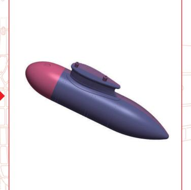
Align the thinner and fatter protrusions on the drop tank with the drop tank head 081-03.
