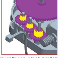
Applying a small amount of grease or lubricant to the gears will help to make them run more smoothly.
