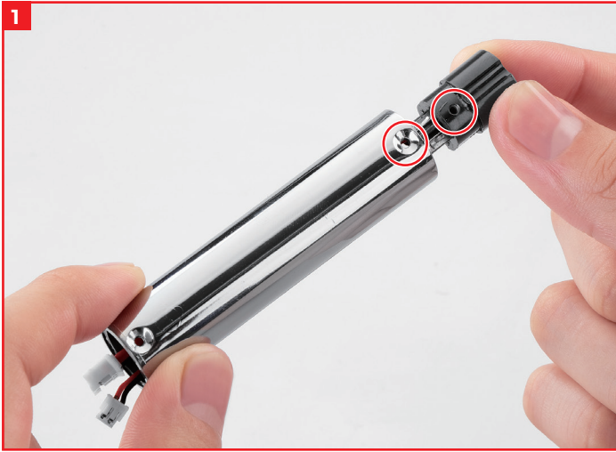
Plug the power connector 085-02 into pipe 085-01 .
