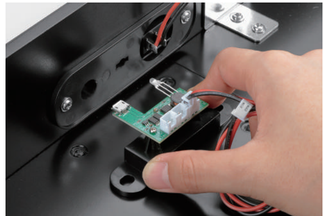
When placing the charging unit on the base plate it's easier to slide it in from the side.
