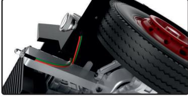
The diagram below shows the LED cable and fog lamp fitted in place.
