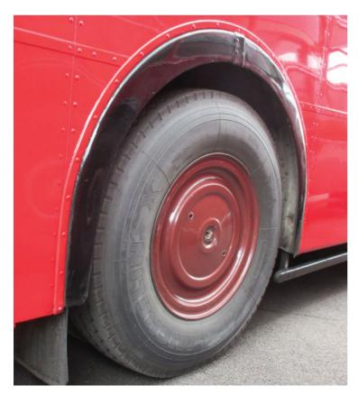
The rear wheel and wheel arch of Routemaster RM1 (left). The mud flap hangs behind the wheel, below the bodywork, to prevent excess mud from splashing up to the suspension mechanism behind the wheels.
