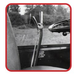
The handbrake is positioned on the nearside of the driver's cab, against the left wall.
