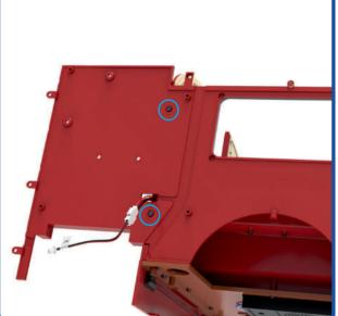
Working from the outside, fix the edge of the rear entrance wall **52A** in place using two **JP** screws. The inset (right) shows the wall in place with the **JP** screws circled in light blue.
