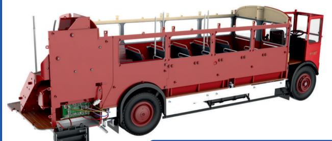
The body of the bus is now fitted to the chassis frame, and the stairs and platform are attached to the back of the bus. The cables have been connected to the circuit board under the stairs (right).
