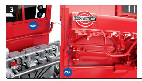
AT THE SAME TIME align the peg on the heating line **40F** against the hole beneath the bonnet on the front wall **47A**. When all these elements are in place, you can start to fix the chassis and body together.
