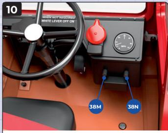
Press the switch **38N** in the driver's cab to check the horn sound. Press the switch **38M** to check the LED lamps on the lower deck ceiling and the headlights and sidelights on the front of the bus, as shown in the insets below.
