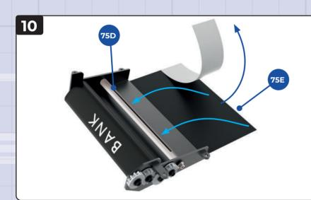
Peel the protective backing off the free end of the blind **75E**. Bring the lower edge of the blind up to align with the black line on the second roller **75D**. When it is accurately aligned, straight and central, fix the self-adhesive strip in place on the roller.
