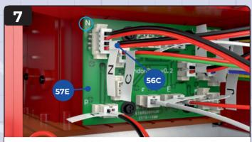
Plug the wide end of cable N **56C**, coming from the roof assembly, into socket **N** on circuit board **57E**.
