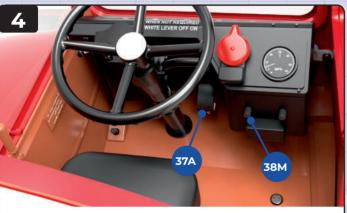
Press switch **38M** in the driver's cab to illuminate the red LEDs on cable O. Press the brake pedal **37A** to see that the LEDs become brighter. These are the rear lights, which also act as brake lights.
