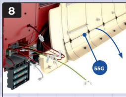
Test that the bells work by pulling the cord on the ceiling of the lower deck (**55G**) and pushing the bells **53D** (inset, below).
