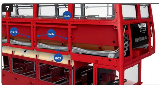
Continue to feed the cable F (**80J**) through the gap between the frame **87A** and the inner wall of the bus, and then behind the frame **87B**, down the right-hand side of the model.
