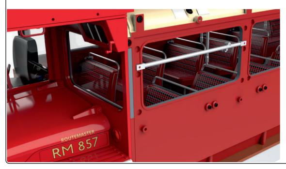
A bar has been fitted to the front window of the lower deck. The section of framework (fitted with windows in steps 1–6) will be fitted in a future stage and hold the bar in place.
