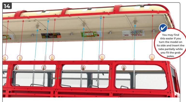
The next step is to fit the roof of the upper deck (see also step 15). Open the windows (green arrows) and align the roof assembly with the framework of the upper deck. As you do so, on both sides of the bus, ensure that the grab
