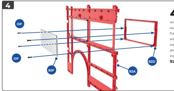
Fit the window frame 92D (with sliding window pane 92E) on to the outside of the left wall framework 92A. Fit the window pane 92F to the inside of the framework, as shown. Fix in place from the inside of the window pane 92F with four OP screws.
