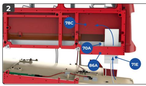
Carefully lift the upper deck slightly, so that you can slip the light panel **71E** in between the outer wall framework **86A** and the ceiling framework **70A**. Ensure that the backing paper is facing away from you.
