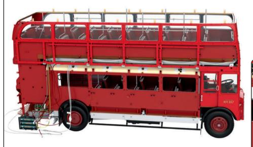
The driver's door has been fitted and an LED has been inserted over the open platform. An outer frame section has been fitted around the front blind.
