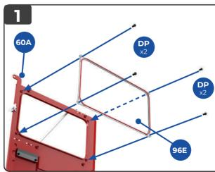
Take the window pane **96E**, supplied with the previous stage, and fit it over the window opening in the platform rear wall **60A**. Fit it on the outside of the wall, with the red rim on the window pane facing outwards. Fix in place with four **DP** screws, supplied with the previous stage.
