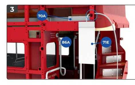
Bring the cable up behind the framework **86A** (circled). Bring the LED panel **71E** through the opening so that it hangs down in front of the framework **86A**. It is advisable to temporarily secure the panel in place with a piece of low-tack tape.
