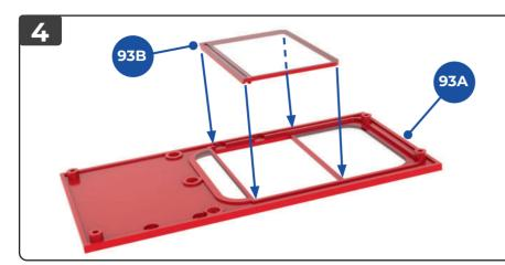
Take the outer door panel of the driver's door **93A** and position it on your work surface as shown. Take the window pane **93B** and position it on the door panel **93A** as indicated. Note the orientation of the ridge on part **93B** (see inset).
