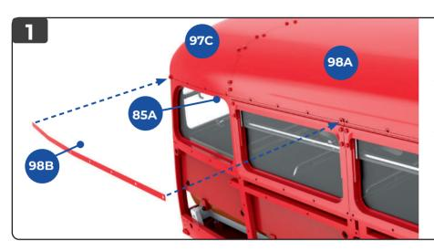
Position the left side strip **98B** along the front left side of the upper deck, covering the edge of the roof panels **97C** and **98A**. Note that one end of the strip is slightly angled at the end – this should be at the front of the model.
