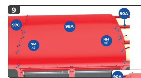
Fix the roof panel **98A** in place, using a total of 23 red **NM** screws: the screws at the front fix into ceiling frame **89A**, and along the rear edge they fix into ceiling frame **90A**. The diagram on the left shows the view from the left-hand side, and the inset below shows the view from the right-hand side.
