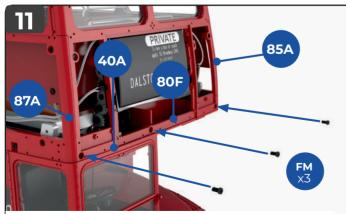
Fix the front framework **80F** to the right wall framework **87A**, the left wall framework **85A** and the cab frame **40A** using three **FM** screws.
