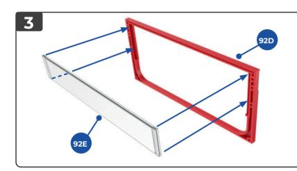
Fit the sliding window pane **92E** into the window frame **92D** so that ridges on the ends of part **92E** fit into the grooves in the frame **92D**. The 'metal' edge of the sliding window goes at the top.
