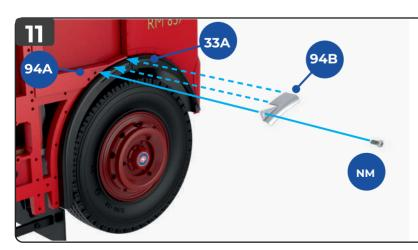
Fit the long tab on the step **94B** between the front right wheel arch **33A** and the right wall framework **94A**, as indicated by the dotted lines. You may need to loosen the screws holding part **94A** in place in order to create space to fit the tab on the step between parts **94A** and **33A**. Fix the step in place with an **NM** screw.
