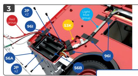
Fix the top edge of the battery box 56B in place with two JP screws (supplied with stage 96). Use two more JP screws to fix the battery box to the rear platform 56A, inserting them from the underside of the rear platform. Use four strips of tape 96I to fix the 'red', 'light blue' and 'yellow' (53K) cables in place. The inset below shows the finished arrangement of the cables.
