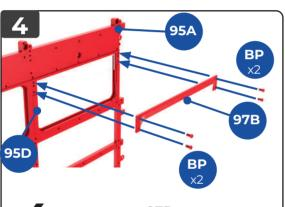
Fit the rain shield **97B** (supplied with the previous stage) against the window frame (**95D**) in the rear right wall frame **95A**. Fix in place with four red **BP** screws.
