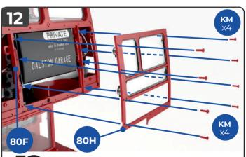
Take the front (blind) frame **80H** (supplied with stage 80) and fit it against the front frame **80F**.
