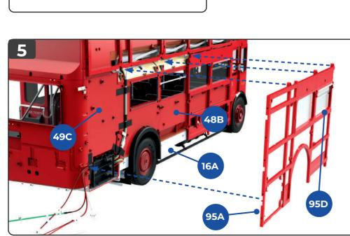
Position the right wall framework 95A aganst the rear right wall of the model. The tabs along the top of part 95A fit into recesses in the upper wall framework. At the right rear corner, the cables running across part 49C fit into a recess in the framework 95A. At the base of the framwork, screw holes align with holes in the rear chassis frame 16A.
