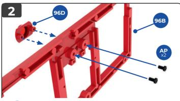
Fit the screw sockets on the bracket **96D** into the recesses in the rear frame **96B**. (Only the lower part of the frame is shown here.) Fix in place with two **AP** screws.
