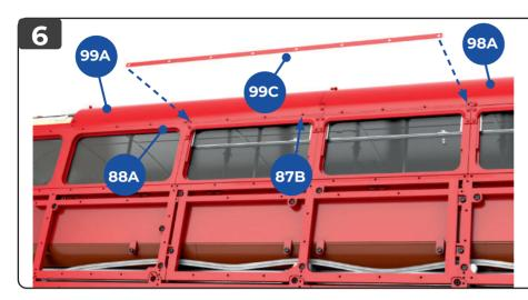
Fit the right side strip **99C** (marked Al89M on the back) to the right wall frameworks **88A** and **87B**, covering the edge of the roof panels **99A** and **98A**.
