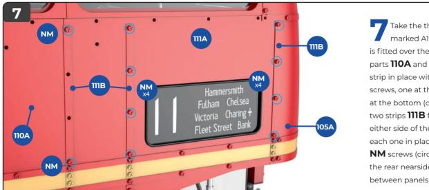
Take the three strips 111B, marked Al97B. The first one is fitted over the seam between parts 110A and 111A. Fix the first strip in place with two red NM screws, one at the top and one at the bottom (circled). The next two strips 111B fit vertically on either side of the blind panel. Fix each one in place with four red NM screws (circled). The strip at the rear nearside covers the seam between panels 111A and 105A.
