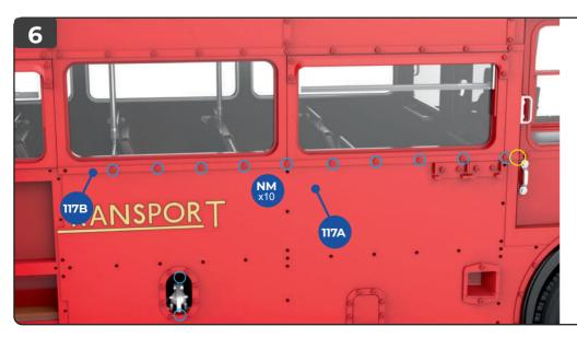
Take strip 117B, marked A163, and fit it along the top of panel 117A, checking that the screw holes are aligned. Note that at the front, the strip extends to the driver's door opening (circled in yellow). Fix in place with ten red NM screws (circled). They go through the strip and the panel, into the frame beneath. Leave the hole at the left-hand end free for the moment.
