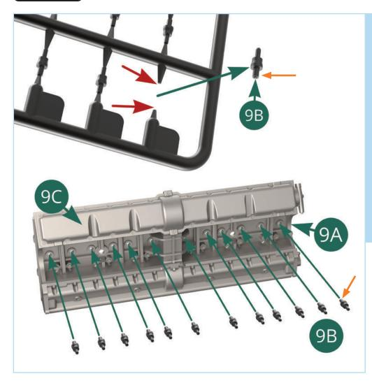
Remove twelve **spark plugs (9B)** from their frame at the points indicated with red arrows. Push them into the **right cylinder head (9A)** using the wider lug (orange arrows) as shown.
