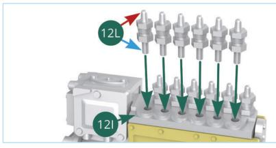
Push the other six injector nozzles into the remaining holes on the fuel pump.
