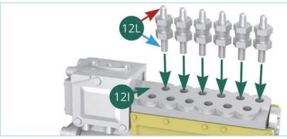
Push six of the injector nozzles into the **fuel pump outer body (12I)**. Note the rounded end (red arrow) points up and the flat end (blue arrow) fits into the hole when fitting an injector in place.
