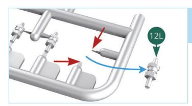
Using sprue cutters, carefully detach twelve **injector nozzles (12L)** from their sprue at the points indicated by the red arrows.
