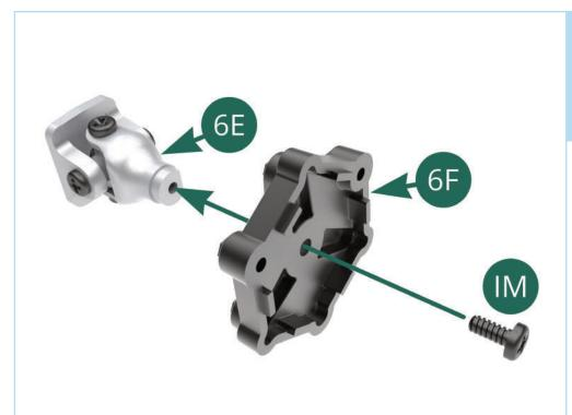
Fit the inner flex disc (6F) onto the transmission flexible joint (6E) as shown and secure it in place with an IM screw.
