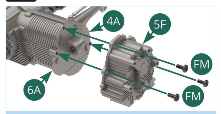
Take the **gearbox rear cover (5F)** from Stage 5 and place it onto the end of the gearbox cover assembly (**4A** and **6A**) as shown. Secure the rear cover using three **FM** screws.
