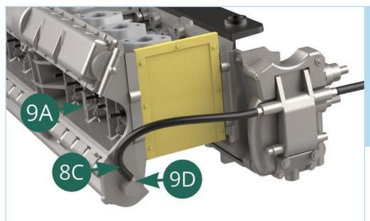
Connect the loose end of the oil hose (8C) on the engine block onto the lug at the end of the exhaust cam cover (9D) as shown.
