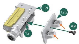
Note the wide holes (orange arrows) when aligning the fuel pump base.
