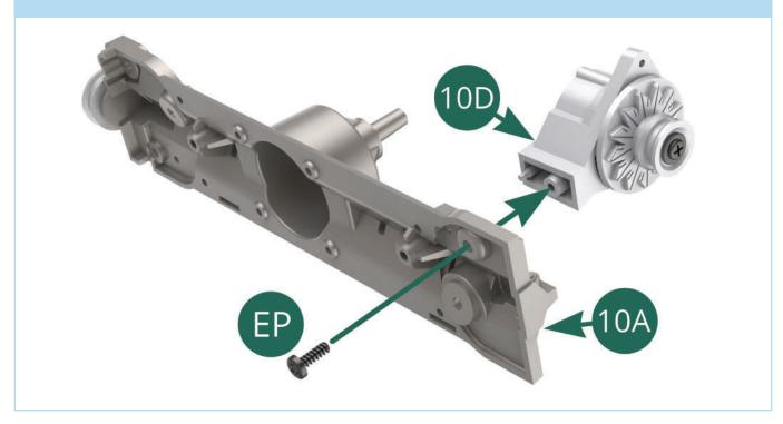
The second alternator fits at the other end of the crankcase top in the same way. Drive an **EP** screw through to attach it.
