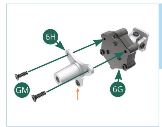
Take the cardan socket (6H) and align it with the outer flex disc (6G) as shown. Note the false 'screw' (orange arrow) on the socket is opposite the previous false 'screw'.
