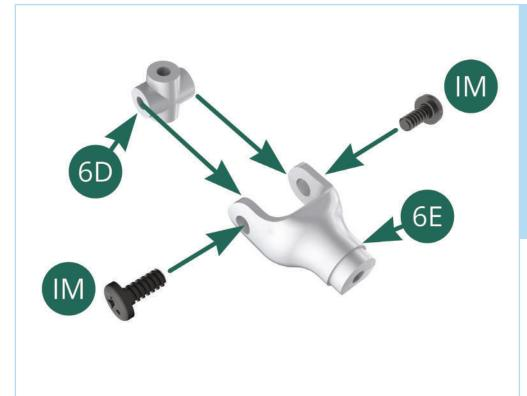
Take the **crosspiece** (6D) and fit it into the transmission flexible joint (6E) as shown. Secure the parts with two IM screws.
