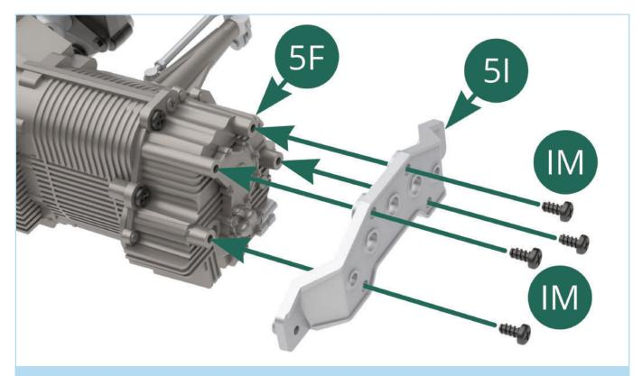
Next take the **exhaust pipe bracket (5I)** supplied in Stage 5 and fit it onto the **gearbox rear cover (5F)** as shown, then attach it using four **IM** screws.
