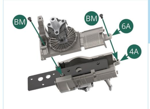
Position the left gearbox cover (6A) onto the right gearbox cover (4A) from Stage 4 and connect the two parts together using two of the BM screws.
