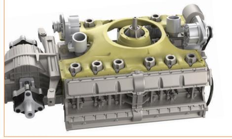
Eight of the air intake brackets and the two distributor bases have been installed onto the engine.
