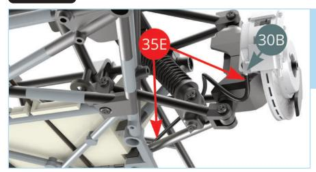
Take the shorter **right brake hose (35E)** and fit one end of it onto the small pin located under the right **brake piston cover (30B)**. Pass the other end around the shock absorber.
