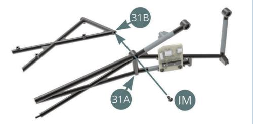
The tubular frame assembly, made up of the frame parts and wiring board, should look like this.
