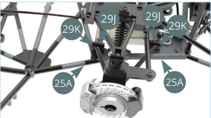
Check that the two **lower control arm brackets (29K)** are located properly in the holes of the **chassis (25A)**.
