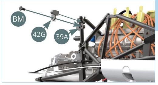
Push the **bracket** (42G) into the **right side frame (39A)** as shown then secure with a **BM** screw.
