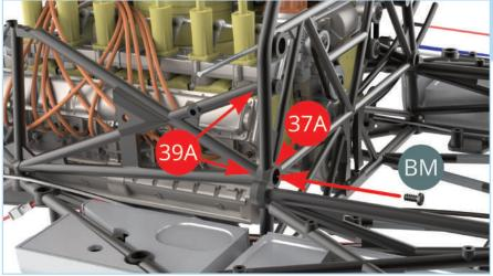
Fix the frame to the central partition using a **BM** screw.
