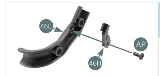
Place the support bracket (46H) onto the transmission cooling line (46E) and secure it using an AP screw.
