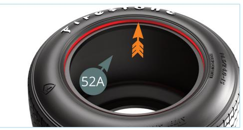
The deepest bead (2 mm) of the tyre is indicated by the green arrow. Locate the side with the deepest bead for fitting the outer rim into the tyre.
