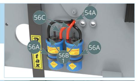
Fit the 95mm lengths of black cable (56B-2) to the pins in the middle of the ignition coils (56A) as shown, then feed the ends of the cables through the middle and right openings in the cabin bulkhead (54A).
