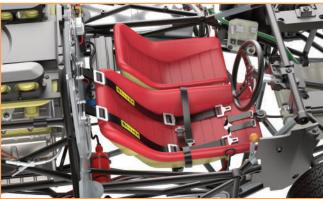
The passenger seat and the driver seat have been fixed to the chassis.
