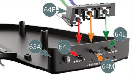
Mount the **instrument panel (64E)** in place, then secure it to the **dashboard (63A)** using two **AP** screws.
