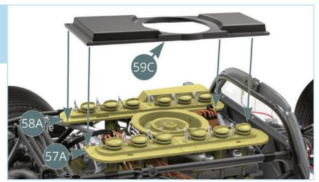
Secure the cover using five **LP** screws as shown.
