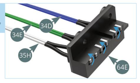
Bend the black sections of the cables of the horn switch (green) (34E), light switch (white) (35H) and engine sound switch (blue) (34D) to fit around the two fixing holes in the button housing (64E), as indicated by the blue arrows.
