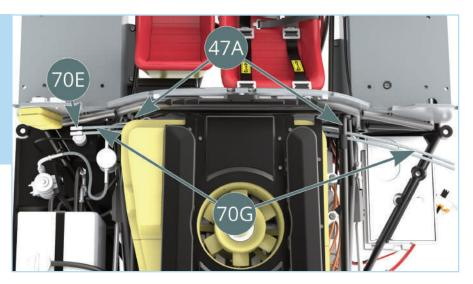
Bend the **fuel lines (70G)** and fit the **connectors (70E)**, highlighted red, onto the pins of the **fuel manifold (70B)**.
