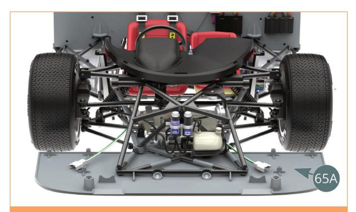
The dashboard and front floor panel have been mounted onto the chassis.
