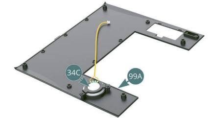
The speaker should look like this once it has been fitted onto the bottom panel.
