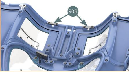
The hinge clamps should look like this once fastened to the front body.
