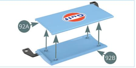
Align the centre spoiler with the **rear hood (90A)** as shown. Fit the holes of the **centre spoiler bottom (92B)** over the indicated screw holes of the rear hood.
