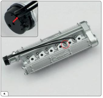
Now fit one of the B cables onto the cable connector adjacent to the previous one (inset). Push the other end of the cable into the next spark plug (circled).
