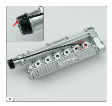
Next take one of the spark plug A cables and push the end onto the topmost cable connector on the distributor cap (inset) and the furthest spark plug (circled).
