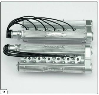
Repeat steps 2 to 10 for the right cylinder head from Stage 10. The two cylinder heads should look like this once finished.
