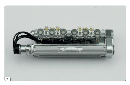
This image shows how the spark plug cables lead behind the carburettors on the cylinder head.
