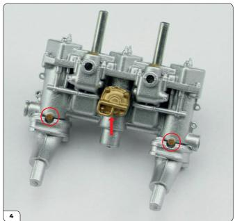
Press the manifolds with two recesses into place on the carburettor as shown, so that the golden pins of the carburettor (circled) sit in the recesses. The curve of the manifolds should lead towards the same side as the golden part (arrow).
