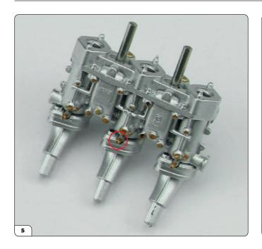
Now install the manifold with one recess by fitting it onto the middle as shown. The recess houses the protruding golden pin (circled).
