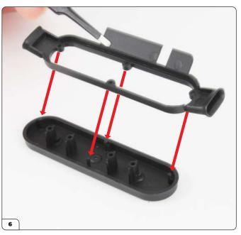
Align the air filter box cover with the air filter box as shown. Note the pins and their corresponding holes (arrows).
