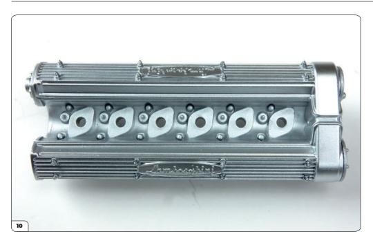
The left cylinder head should look like this with both covers and all of the bolts installed.
