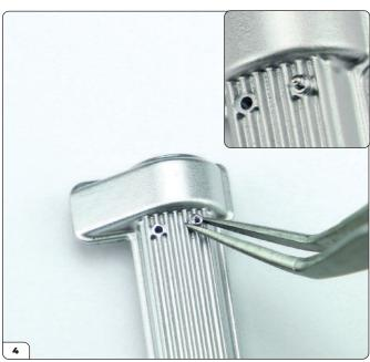
Using pliers or tweezers, carefully grasp a bolt by the ring around it and fit into one of the holes as shown. The long smooth end of the bolt is fitted into the hole, leaving the bolt's hex head visible (inset).
