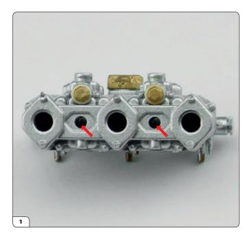
Locate the two smaller holes on the carburettor (arrows), found between the three larger holes.
