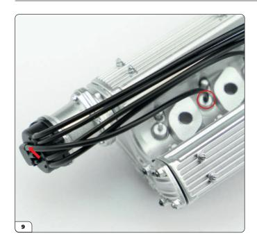
Take one of the E cables and fit it to the topmost connector on the attachment (arrow) and the furthest spark plug (circled).
