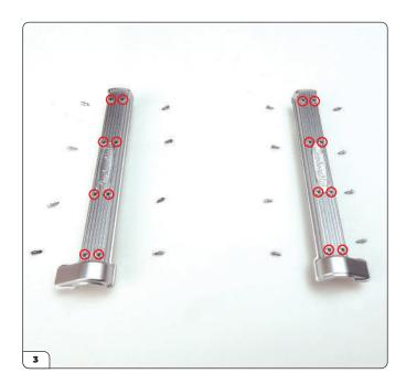
Take the two cam shaft covers and lay them on your work surface as shown. There are eight holes (circled) in each cover into which the bolts will be inserted.
