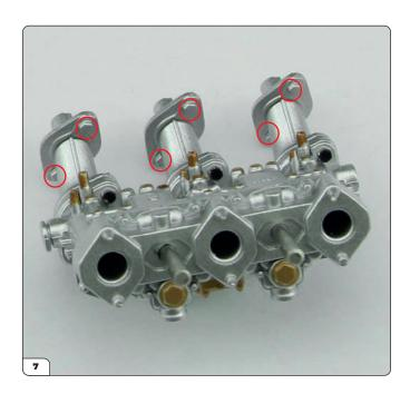
Fit the three shims onto the ends of the manifolds so that the nuts (circled) face towards the carburettor as shown.
