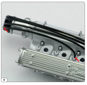
Then take one of the D cables and fit onto the indicated connector and spark plug (arrows).
