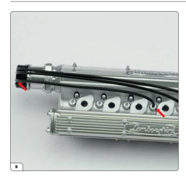
Fit one of the C cables into the next connector and spark plug in sequence (arrows).
