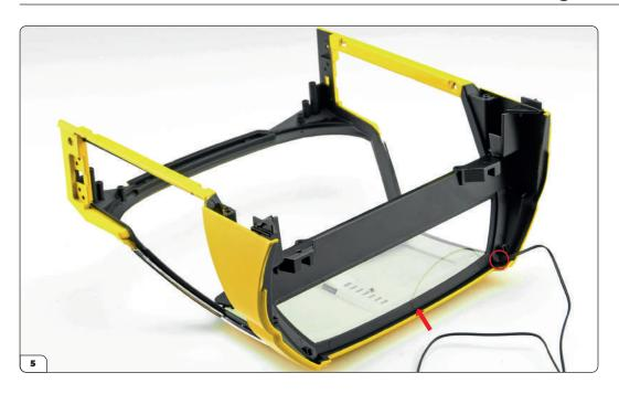
Carefully push the window so that it fits into the recess and is flush with the body (arrow). Note the inner light cable protruding from the notch (circled).
