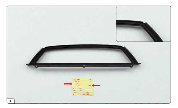
Next take the rear window support and double-sided tape (supplied with the previous stage). Lay the support with the recessed area facing upwards (note the appearance of the corner, inset). The double-sided tape sheet has six straight pieces and two curved pieces (arrows).
