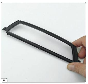
Remove the white backing from the double-sided tape strips. Press the window into the support, starting with one corner. Once in place, use a microfibre cloth to carefully push the window down on the tape to ensure it adheres completely.
