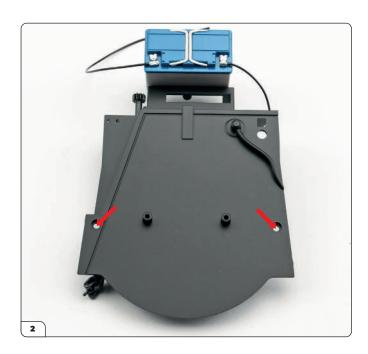
Take the front frame cover which was assembled in the previous stage. The two holes (red arrows) fit over the left and right holes highlighted in the first step.
