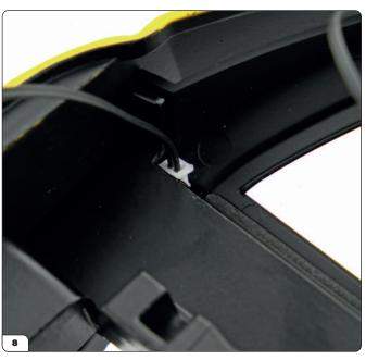
Using tweezers, grasp the connector and push the inner light cable through the hole highlighted in the previous step.
