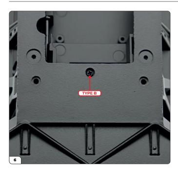
Turn the assembly over and use a Type B screw (supplied with Stage 56) to secure the point underneath the battery to the front frame.
