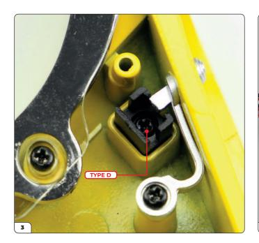
Secure the housing in place using a Type D screw.
