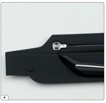
Push the pin of the handle through the hole and fit it in place.
