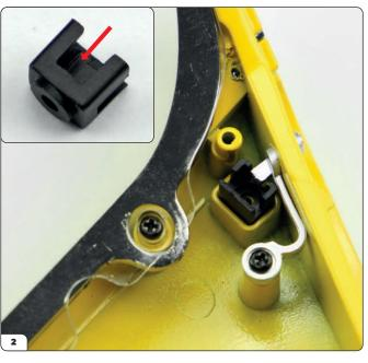
The light switch housing has an opening on the side to accommodate the light switch button (inset, arrow). Fit the housing into its seat so that the switch fits through this opening as shown.
