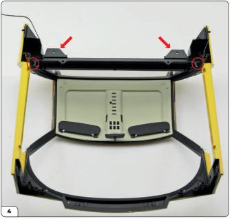
Next you'll mount the cross frame and rear window into the central body. Align the frame so that the highlighted trapezoid structures (arrows) face outwards, then carefully lower the frame into position. The holes at each end (circled) should sit over the corresponding screw columns of the body. Make sure the inner light cable remains in place so that it protrudes through the notch (see step 5).
