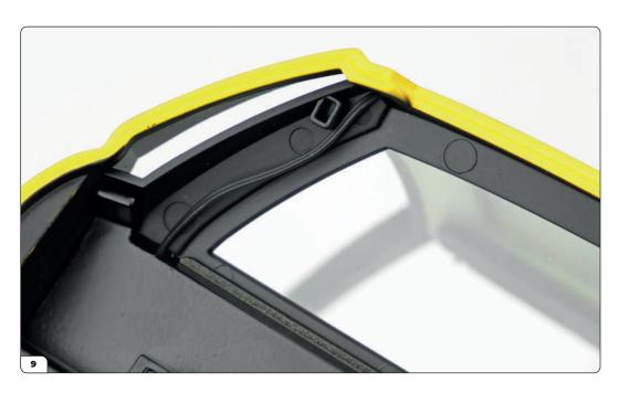
Once the connector is through the hole, pull until the cable is flush with the rear window as shown above.
