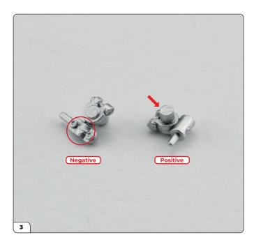
The terminal posts (supplied with Stage 54) are different from each other. Lay them on the work surface as shown and identify the postive and negative post. The negative post has two screws on a wider base (circled). Each one has a thick pin for fitting it into the battery (arrow).
