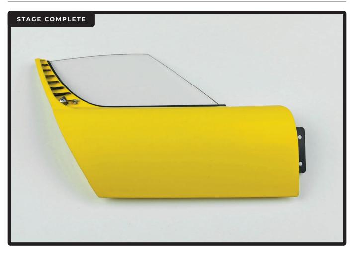
In this stage the light switch is installed then the right door panel is fitted. The cladding panel can be put aside for now, it will be attached in the next stage.
