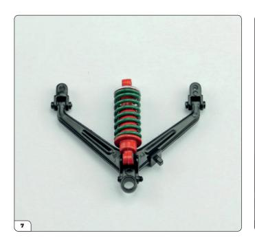
Fit the front shock absorber in the appropriate housing located on the upper face of the wishbone arm as shown.
