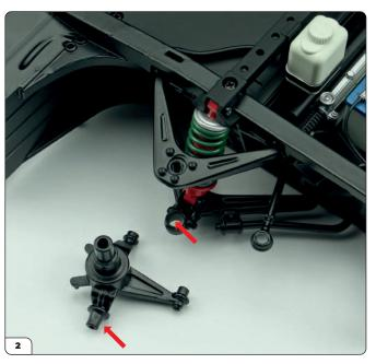
Retrieve the front frame assembly and place it on the work surface with the right-hand side facing you. Align the front right wheel hub with it as shown. Note the column and hole indicated by the arrows.
