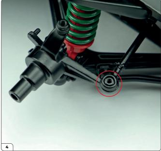
Connect the steering arm to the wheel hub (circled).
