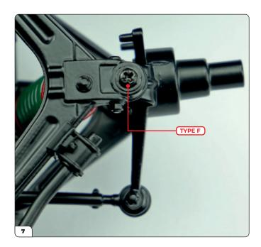
Turn the assembly over and fix the bottom of the wheel hub using a type F screw. Again, don't overtighten the screw.
