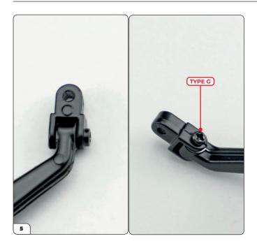
Fit the bracket onto the end of the wishbone arm as shown then secure it using a Type G screw.
