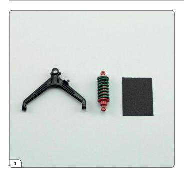
Take the front left lower wishbone arm and front shock absorber supplied with Stage 60, along with one of the pieces of sandpaper supplied in this stage. You can also use a fine flat file in place of the sandpaper for the next steps.
