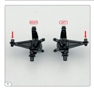
Take the two front wheel hubs from the previous stage. Place them on the work surface as shown and identify the left from the right hub. Note the connection points for the steering rack (arrows) are facing upwards in the photo.
