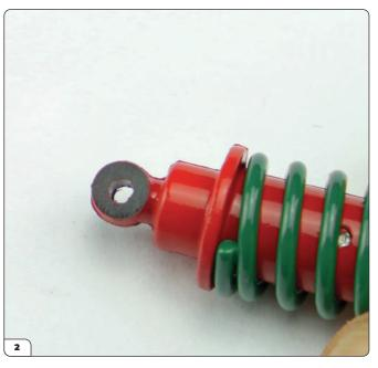
Remove excess paint from the shock absorber using a flat file or the sandpaper supplied with Stage 61 if necessary.
