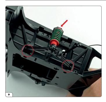
In the same manner as before, fit the wishbone arm brackets into the two square-shaped holes located at the base of the left-hand side of the frame (circled) and insert the upper attachment point of the shock absorber into the end of the frame reinforcement crossbar (arrow) at the same time.
