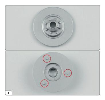
Take the outer half of the front left brake disc supplied with Stage 64 and place it on the work surface. Turning it over, you will see three mounting pins (circled).
