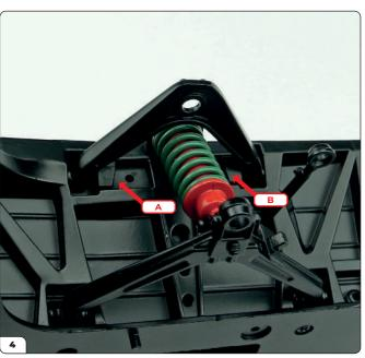
Position support A in the housing to the left of the shock absorber. Then insert support B to the right of the shock absorber as shown. We recommend using a pair of tweezers to push the supports in place.
