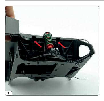
Take the front frame assembly and locate the seats for the ends of the front right upper wishbone arm next to the shock absorber (arrows) on the right side of the frame.
