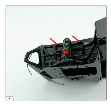
Take the front frame assembly and locate the seats for the ends of the front left upper wishbone arm next to the shock absorber (arrows) on the left side of the frame.
