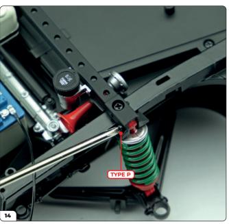
Repeat for the shock absorber on the other side using another Type P screw (supplied with Stage 61) as shown.
