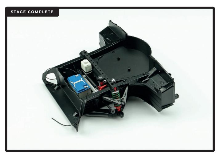
Next you'll fit the right upper wishbone arm and torsion bar in the same manner as before using the parts supplied with Stage 63.
