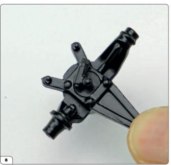
Press the left angle drive into the centre of the hub, orienting it in the direction shown in the photo.
