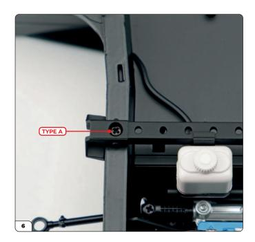
Fix one side of the crossbar to the frame using a Type A screw (supplied with Stage 59).
