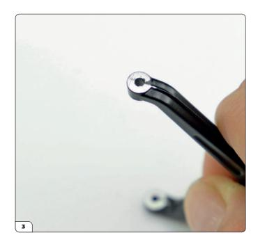
Remove excess paint from the ends of the wishbone arm using a file or the sandpaper supplied if necessary.
