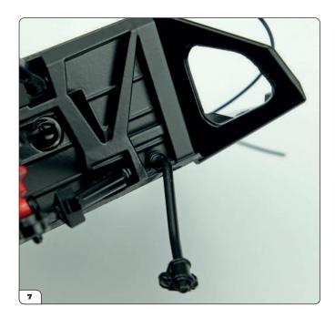
Then take the torsion bar from Stage 63 and insert the pin located on the curved end of the piece into the hole identified in step 6.
