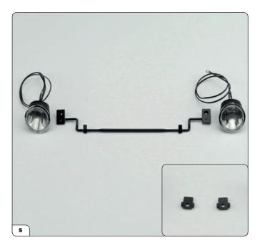
Place the headlight support (supplied with Stage 79) on your work surface, then align the two headlights with it as shown.
