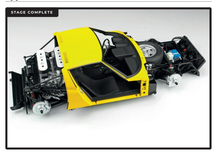
With the front and rear frames installed into the body, you can now fix the left and right doors onto the main assembly. Then you'll connect the switches from the doors to the circuit board.
