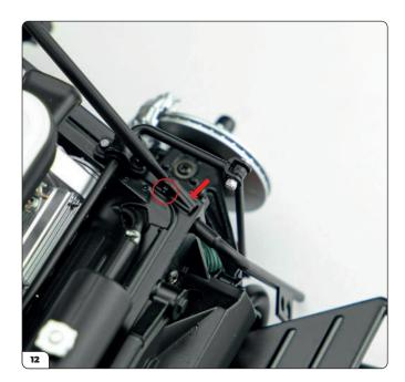
Carefully flex the right rod from the middle and guide its triangular end into the slot located on the rear frame (arrow). Note the nut facing inwards (circled).
