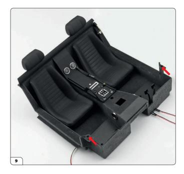
Retrieve the cockpit assembly and place it on your work surface. There are two holes on the front for fixing it to the body (arrows).
