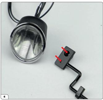
Each end of the support has a bracket with a small and large hole (arrows) for mounting the headlight.
