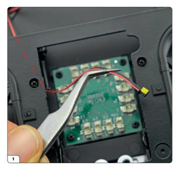
Take the indicator switch coming from the steering wheel column, which has a black plug with a yellow pad. Pass it under the crossmember of the frame (dashed line).
