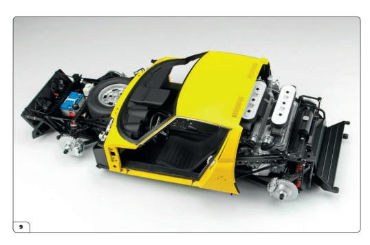
The assembly should look like this once the rear frame has been fixed to the body.
