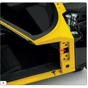
Starting with the right-hand side, locate the square hole in the housing for the door hinge (arrow).
