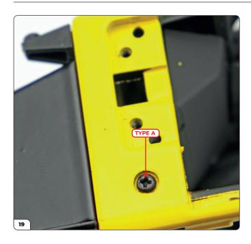
Continue to fix the assemblies together with a third Type A screw in the outer hole at the base of the driver's side door hinge housing. The screw should sit flush inside the recess.
