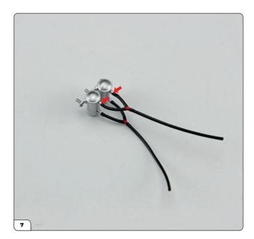
Push one pair of the short tubes onto the top pins of the fuel pumps (red arrows). The other pair fits onto the bottom pins as shown.
