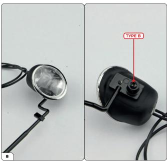
Mount the other headlight in the same manner and secure it using a Type B screw.
