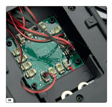
Plug the interior light into connection 16 (arrow).
