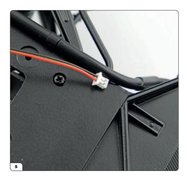
Take the instrument panel LED wire, which is white with red/black cables, and route it under the crossmember.
