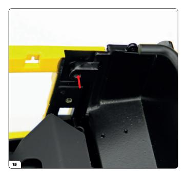
Make sure that the holes in the base of the door hinge housings (arrow) line up on both sides of the components.
