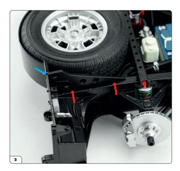
Repeat on the other side of the frame to fit the right reinforcement plate in place.
