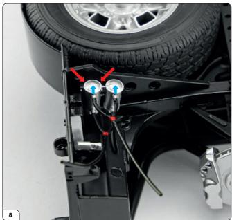
You can now mount the fuel pump bracket onto the right-hand frame reinforcement plate. To do this, insert the pins of the pump bracket into the two holes on the plate (red arrows). Note that the rounded ends (blue arrows) of the fuel pumps are oriented upwards.
