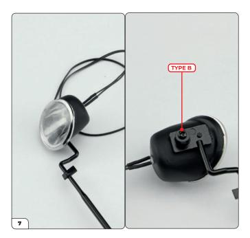
Mount one of the headlights onto one end of the support, then secure it using a Type B screw (supplied with Stage 79).
