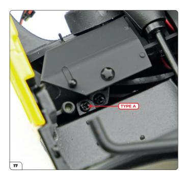
Once you have ensured that the front assembly of the chassis is positioned correctly, you can fix everything with four Type A screws. Start inserting the first one in the slot on the driver's side, located next to the dashboard fixing point.
