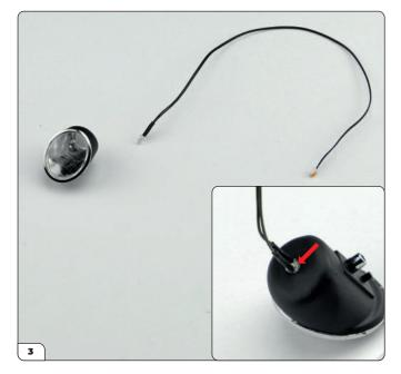
Take one of the headlight LEDs (supplied with Stage 79) and insert the bulb end into the hole at the back of the housing (inset). The fit may be tight, we recommend holding behind the bulb with a pair of tweezers to firmly press it into place.
