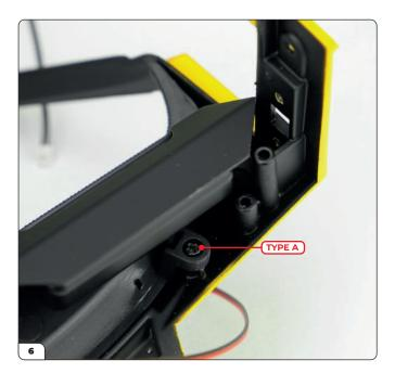
Secure the right-hand side of the dashboard with a Type A screw.
