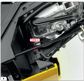
Drive another of the Type A screws into the trapezoid-shaped connection on the passenger's side.
