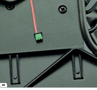
Plug the accelerator switch into connection 3 (arrow).
