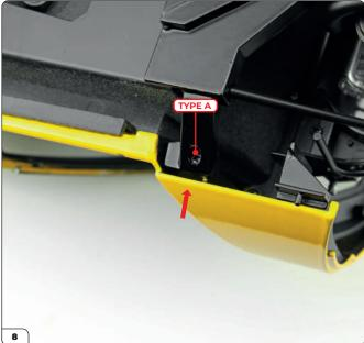
Returning to the driver's side, fasten the outermost connection point with a Type A screw. You may need to apply some pressure to the body (arrow) to ensure the holes are aligned as you drive the screw in.
