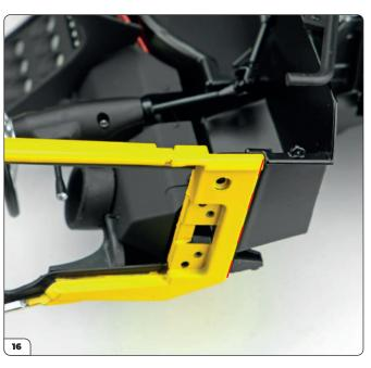
Also check that the front frame assembly is properly seated by checking alignment with the edge of the body, as shown by the dashed line.
