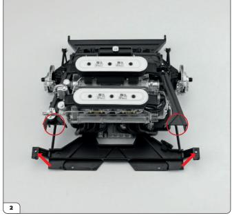
The first part of this stage will be fitting the rear frame into the body. Take the body assembly and locate the four fixing points: the two trapezoid-shaped protrusions along the cross frame firewall (circled) and the two triangular plates underneath them (arrows).
