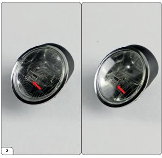
Press one of the lenses into the headlight housings as shown. Note the orientation of the pattern on the lens (arrow).
