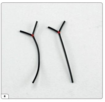
To get a good fit, try twisting the tubes between your thumb and finger as you press them onto the fitting.
