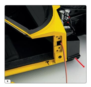
Thread the plug for the door switch through the square hole and through to the lower part of the front frame (arrow – see step 4).
