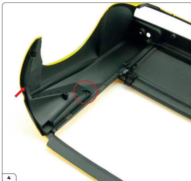
Insert the tab on the left bulkhead into the hole indicated in the previous step (circled). At the same time, insert the pin on the fin into the hole at the edge of the body (arrow). Push firmly until the bulkhead is flush with the body.
