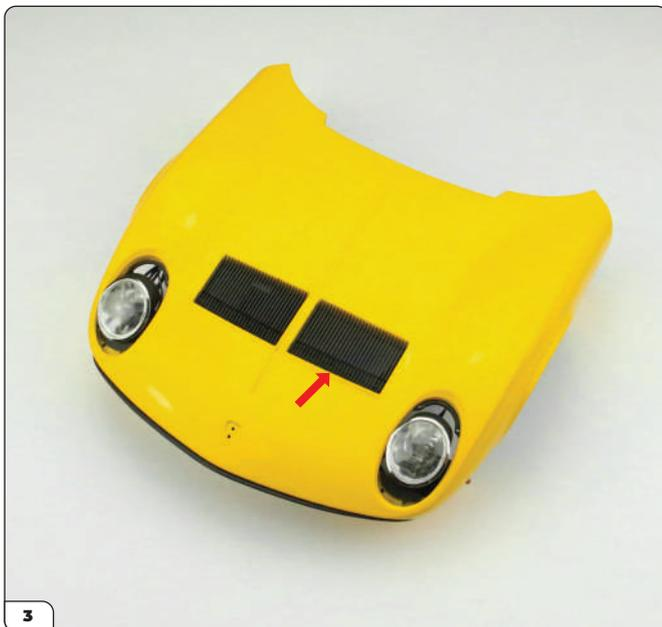
Fit the grille into the left-hand opening so that the large end of the spring is pointing towards the front (arrow).
