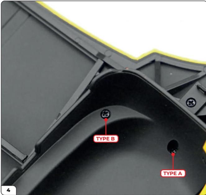
To fix the wheel arches in place, you'll need the Type A and Type B screws supplied with Stage 85. Secure the two fixing points at the rear of the right wheel: start by first driving a Type A screw into the hole inside the well, then drive a Type B screw into the hole in the inner ridge, as indicated.
