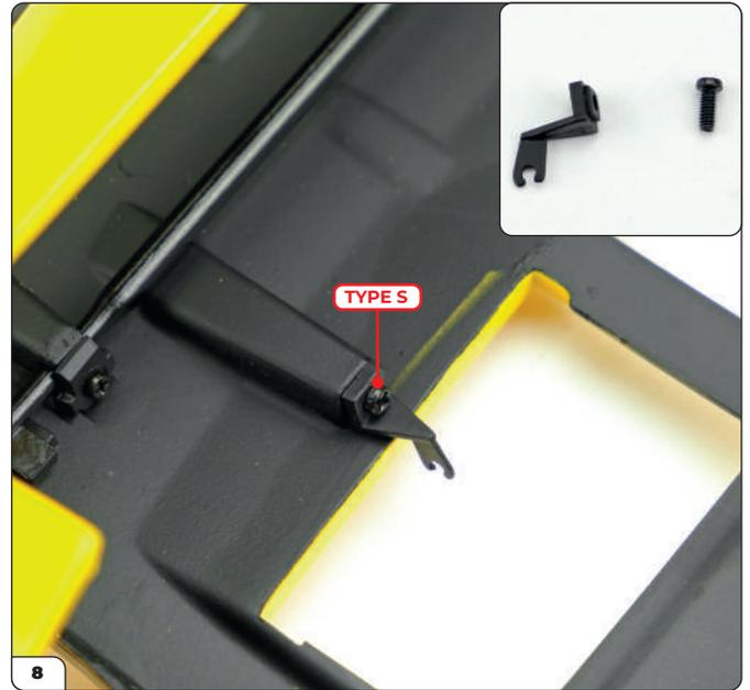
Now take the bonnet grille support and a Type S screw which were supplied with Stage 81 (inset). Position the support on the perforated column located inside the front body near one of the rectangular openings, then fix the holder with the Type S screw as shown. If it is difficult to keep the part in place, you can also drive the screw partially through the grille support, then position it and tighten the screw.
