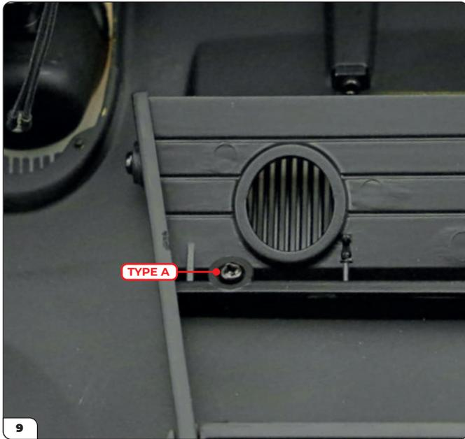
Start by fixing one side of the structure using a Type A screw (supplied with Stage 85).
