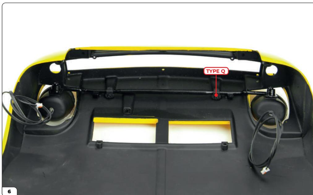
Fit the other support plate to the remaining slot in the same way and secure using a Type Q screw.
