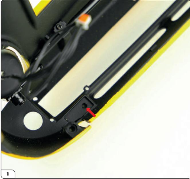
Take the front body and place it upside down on your work surface. Inside the front part, along the lower edge, there are two rectangular recesses (one on the right and one on the left) with a hole each, as shown by the arrow. These openings are the seats for the two bonnet support brackets assembled in the previous stage.
