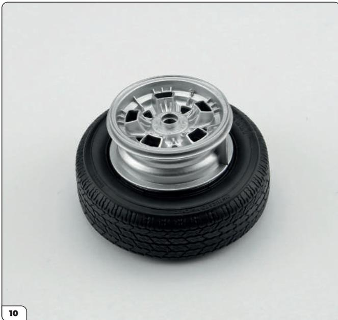
As you did with the previous wheels, insert the rim into the tyre and press it inside until the lip of the rim is flush with the edge of the tyre.
