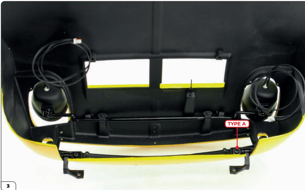
Fit the right support bracket in the same way and secure it using a Type A screw.
