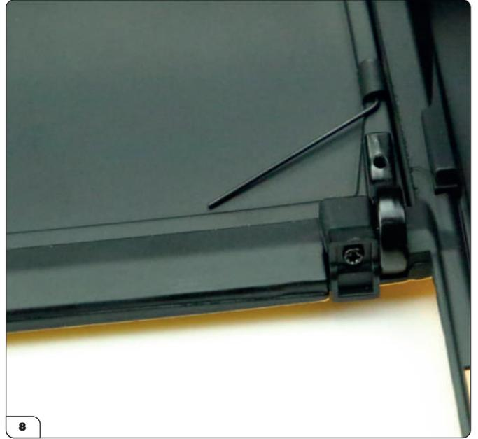
Carefully turn the rear body over again with the boot lid in position. Fit the pin in the right hinge into the hole of the boot lid so that the screw holes align, as shown in the photo. Repeat for the left hinge.
