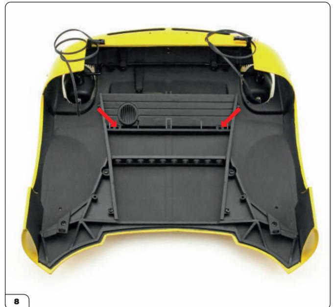
Lay the front body upside down on your work surface then fit the structure into place. Check that the screw holes are aligned (arrows).
