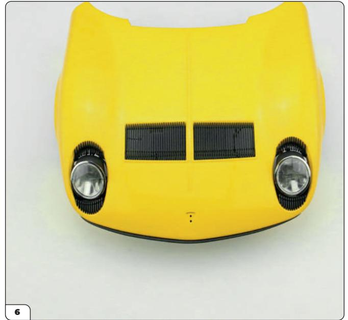
Firmly press the pins of the headlight eyelashes into the holes.
