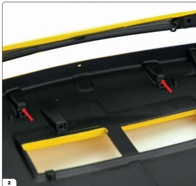
Locate the two slotted supports (arrows) towards the front which will be used for positioning the headlight support.
