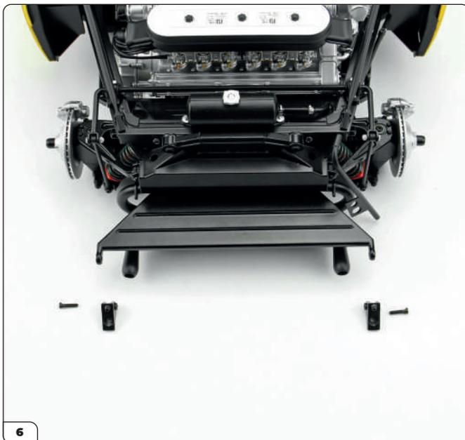
Now take the main body assembly and place it with the rear facing towards you. Take the rear bonnet hinges and 2x Type G screws (supplied with Stage 81).
