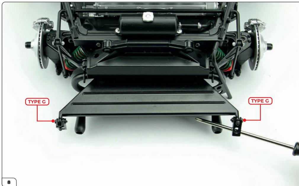
While gripping the hinge tightly, secure each one in place by driving a Type G screw from the outside towards the inside. The hinges should be able to move freely once secured.
