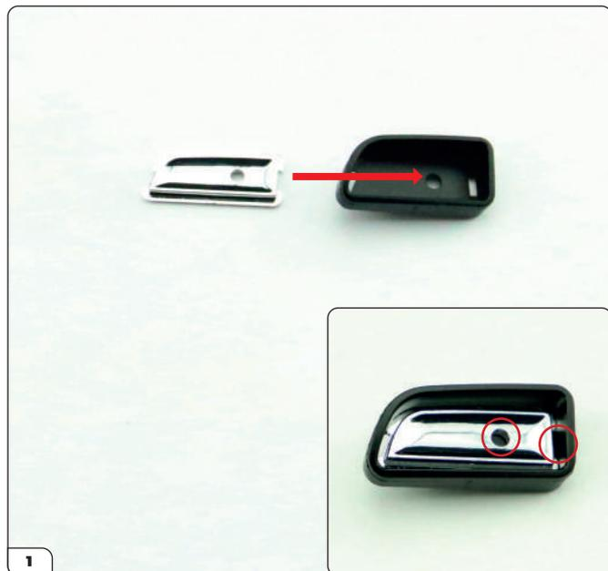
Retrieve the left rear light reflector and housing which were supplied with Stage 89 and align them as shown. Fit the reflector into place inside the housing, making sure the round and rectangular holes are aligned (inset, circled).
