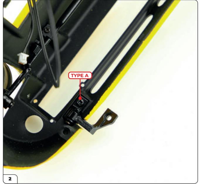
Take the left bonnet support bracket and fit it into the rectangular recess. The arm of the bracket should be facing inwards as shown. Secure in place using a Type A screw (supplied with Stage 81). Ensure it sits properly in the recess and the screw is fully tightened.
