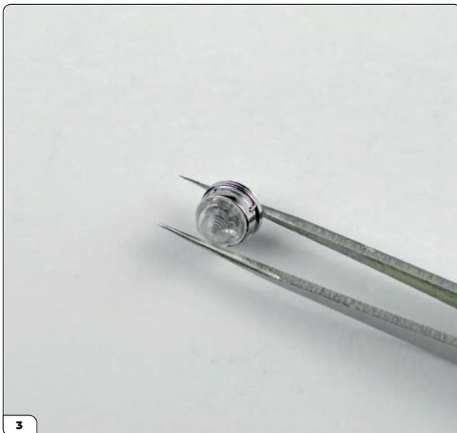
Align the protrusions and recesses then press the parts together.
