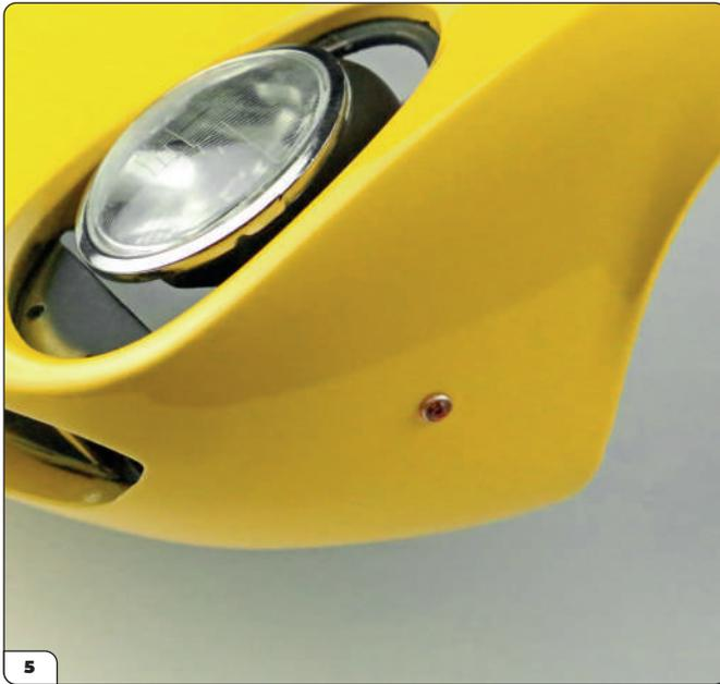
Press the long end of the indicator into the hole on the front body. The indicator is angled to fit flush with the body, inserting it partially and rotating it around to find the correct angle before pressing into place.
