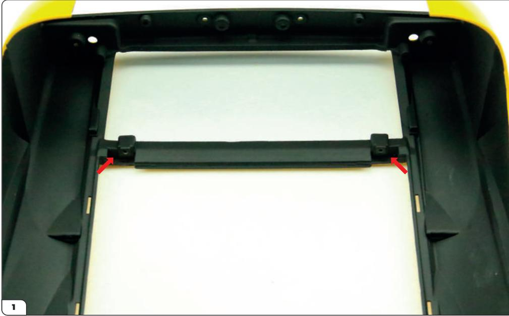
Take the rear body (supplied with Stage 88) and place it upside down on your work surface. To avoid scratching it, you may wish to place it on a cotton or microfiber cloth. Note the two recesses for fitting the hinges (arrows).
