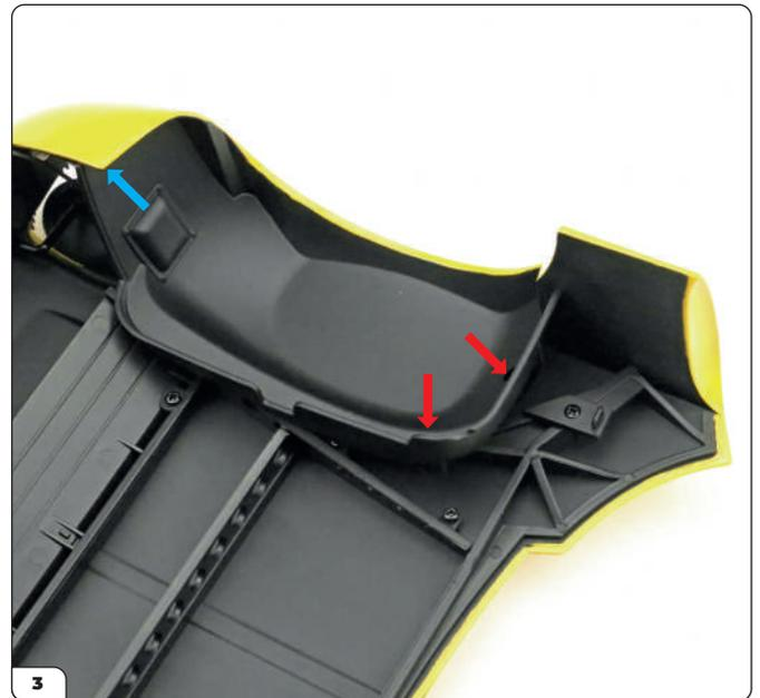
Move the left headlight LED wire out of the way, then mount the left wheel arch into place in the same way, checking the holes (arrows) are aligned.
