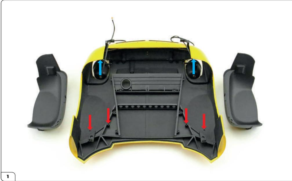
Retrieve the left and right front wheel arches which were supplied in Stages 82 and 83. Place the front body assembly on your work surface and align the two wheel arches with it as shown. Note the holes in the front body assembly for mounting the bulkheads (arrows). The holes indicated by the blue arrows are located underneath the lip of the body.
