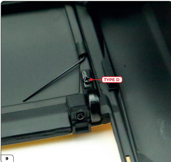
Secure the right hinge to the boot lid using a Type D screw (supplied with Stage 88).
