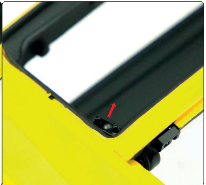
Turn the rear body upright and check that the two hinges move freely up and down, as shown by the red arrows. If the movement is difficult, slightly loosen the fixing screws of the brackets.
