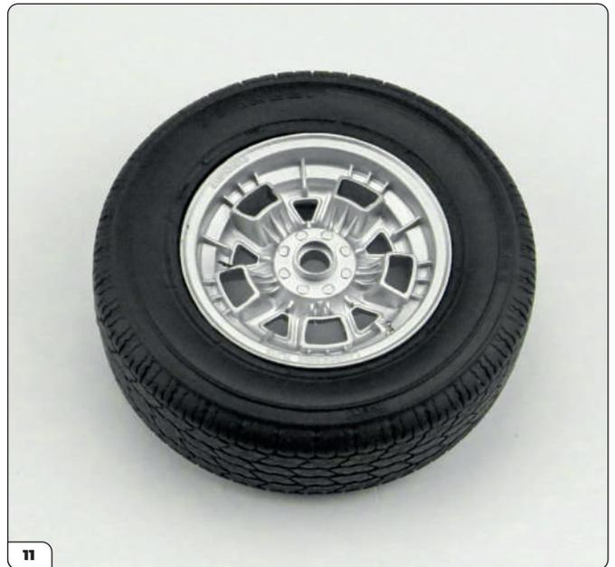
Check that the rim is seated correctly on both sides of the tyre.
