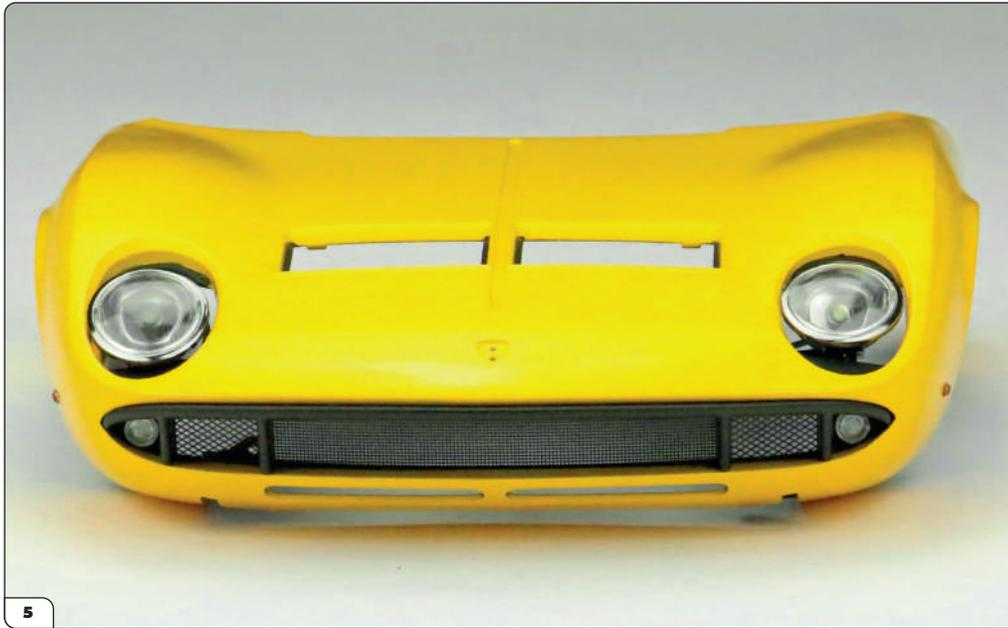
Carefully press the pins of the support into the holes of the front body. Do not put pressure on the grille to avoid damaging it. Once in place, the support will not be flush with the profile of the bonnet, but will protrude slightly.
