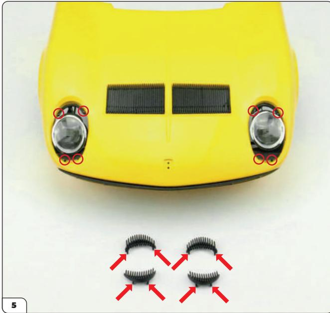
Turn the front body upright and place it on your work surface. Retrieve the left and right headlight eyelashes supplied with Stage 85. Align each pair with the appropriate headlight, noting the difference in the position of the pins for the top and bottom eyelashes (arrows). These correspond with the holes in surrounding the headlights (circled).
