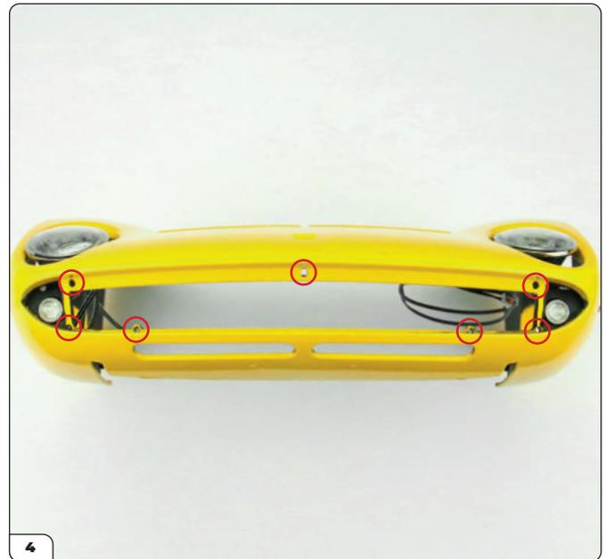
Take the front body assembly and locate the seven holes around the air intake for fitting the support (circled).
