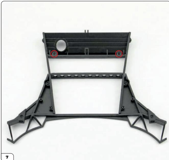
Retrieve the bonnet reinforcement structure and place it upside down on your work surface. There are two screw holes for fixing it to the front body (circled).
