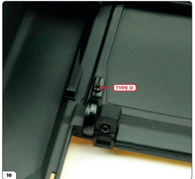
Secure the left hinge with another Type D screw in the same way.
