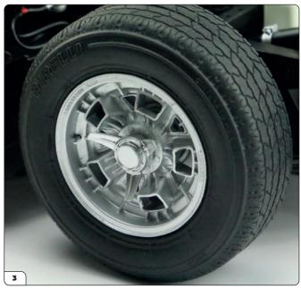
Fit one of the hubs caps over the raised circle of one of the wheels as shown.
