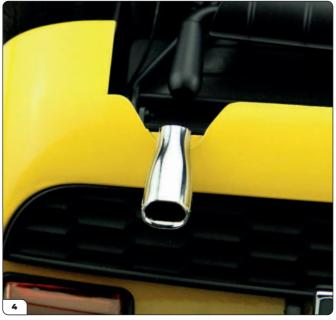
Fit the right tailpipe (marked 'R') into the holes on the driver side in the same way.
