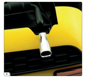
Take the left tailpipe (marked 'L') and fit its pins into the holes on the passenger side as shown.
