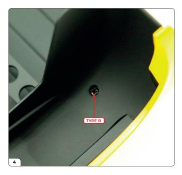
Take a second Type B screw and use it to secure the wheel arch to the body bulkhead.
