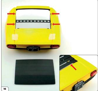
Turn the rear body assembly upright and note the four slots in the recess of the body (arrows) for fitting the rear window grille. Starting at the back end, fit the grille in place and press it firmly into the slots. Note the openings in the grille should face the back end, as shown by the arrow in the inset image.
