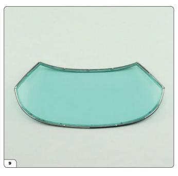
Press the side of the windscreen without the protective film into the trim. Start with the top corners (arrows), then press the screen into the lip, working around the trim slowly so that the screen fits into the curve. Press firmly around the edges to adhere the parts together.
