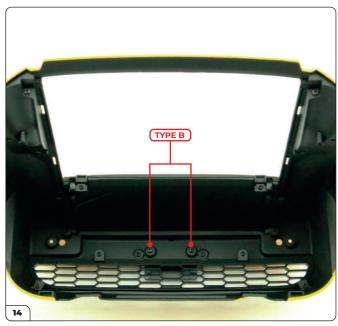
Turn the body around and secure the licence plate using 2x Type B screws (supplied with Stage 91).
