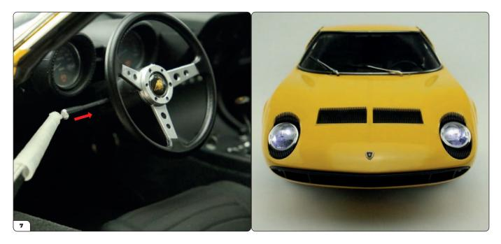
By gently pressing the lever (arrow) inwards, the horn sounds. By slightly pulling the lever towards the steering wheel, the lights on the front and rear lights come on. By repeating the operation, the lights go out. When you are not using the model, always remember to return the switch to the 'OFF' position.
