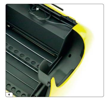
Fit the right rear wheel arch in the same way, pushing the tab into the recess and pressing the arch until all three screw holes are aligned.
