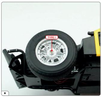
Use one of the Type I screws to fix the wheel in place. Tighten the screw fully and use a drop of oil to lubricate the connection for smoother turning of the wheel.
