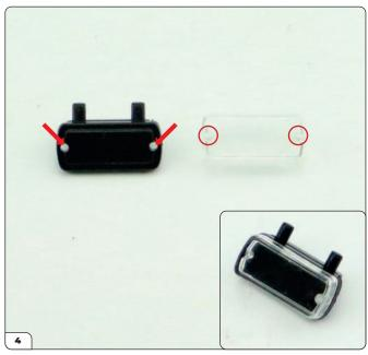
Next take the reverse light glass and support (supplied with Stage 92). The glass has two pins (circled) which fit into the small holes (arrows) of the support. Fit the glass into the light as shown in the inset image.
