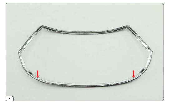
Now take the windscreen trim and lay it on your work surface as shown. The double-sided adhesive tape for fixing the windscreen must be applied to the lip on the inside (concave) part of the windscreen trim, as indicated by the arrows.
