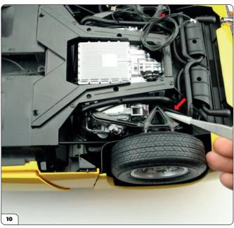
Continue to thread the wire by passing it under the rear lower suspension arm (arrow).
