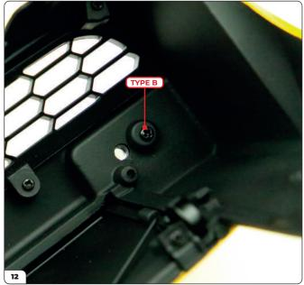
Secure the right taillight housing in the same way using a second Type B screw (supplied with Stage 90).
