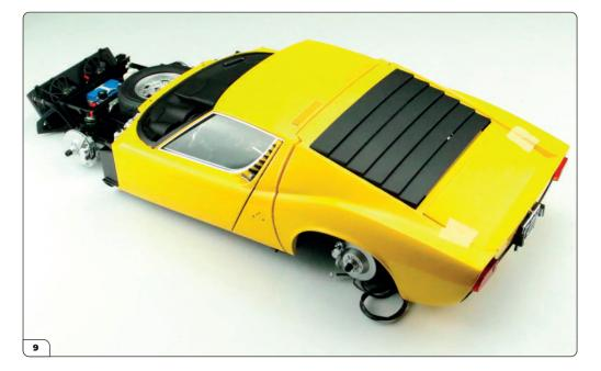
Lay the rear body on top of the central body, starting at the rear and fitting it flush with the roof and B-pillars. Once the fit is flush, use masking tape to hold the rear body in place. Take care that the bodywork does not interfere with the wiring.
