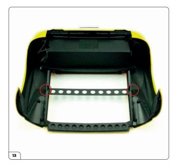
Now take the rear reinforcement structure. Starting with the wide ends, push the structure against the compartment (arrows), then lower the screw holes at the sides into the recesses (circled).
