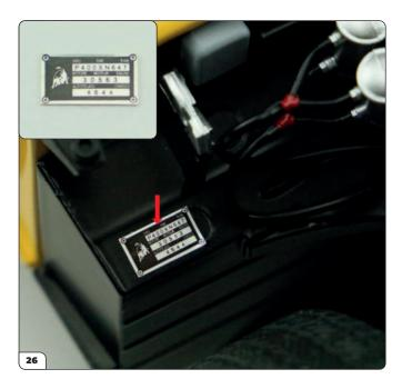
Takle the chassis and engine number plate (inset) and remove the backing paper. Open the front hood and position the plate on the right side of the frame, near to the fuel pumps, as shown (arrow).
