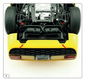
Retrieve the main assembly and place it upside down on your work surface with the rear end facing you. There are two pairs of holes on the rear body (arrows) for mounting the tailpipes.
