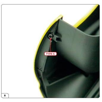
Finally, use a Type S screw to fix the wheel arch to the rear body. Check the holes are aligned first, as you may need to apply pressure while driving the screw in to get the parts to fix.
