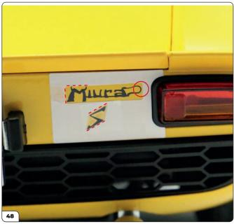
In the same way, peel the 'Miura S' stickers and apply them to the right side using the template. Use the top and left edges of the upper section to align the horns and corner of the 'M', then the angled edges of the lower section to align the 'S' as indicated by the dashed lines. Take care when applying the sticker that the tail of 'Miura' doesn't overlap the template (circled).
