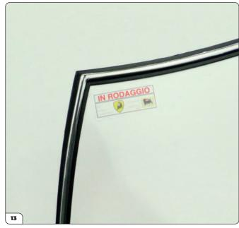
Place the sticker as shown in the windscreen's upper corner on the passenger side. Make sure the area is clean of any dust or fingerprints before sticking.
