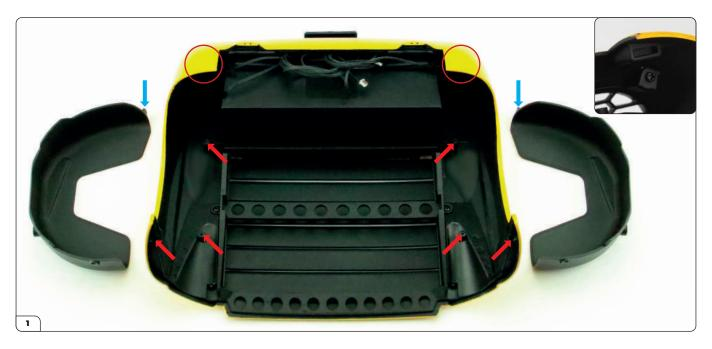
Take the rear body assembly and place it on your work surface upside down, along with the left and right wheel arches as shown. Locate the fixing points: three screw holes (arrows) and a rectangular recess (inset) located underneath the lip of the body (circled) on either side. Note the protruding tabs on the arches (blue arrows) that fit into the rectangular recesses. Be sure to move the wires of the taillight LEDs and the speaker out of the way as shown in the image.
