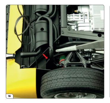
For the left taillight (white plug, black panel), take the end of the wire and guide it along the same path as before. First, pass it underneath the exhaust pipe (arrow).
