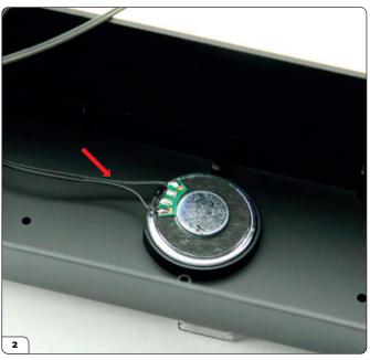
Position the speaker (supplied with Stage 93) in the circular recess inside the boot, so that the wiring leads to your left (arrow), as shown in the image.
