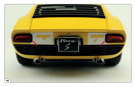
The last few steps are to apply the logos to the rear of the model. First, take the rear logo templates and separate them from their backing. Apply them to the rear body as shown, using the taillights as a guide for fitting them in place (arrows).
