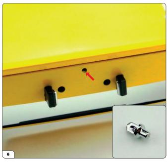
Next take the boot lock (supplied with Stage 90, inset). This has a shaped end for fitting into the hole (arrow) in the rear body located between the licence plate lights.
