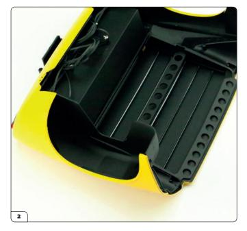
Start to fit the left rear wheel arch by pushing the tab into the rectangular recess, then press the arch in place until all three screw holes highlighted in the previous step are aligned. You may need to apply some pressure to the arch to compress it until it fits in place – be careful not to damage the part.
