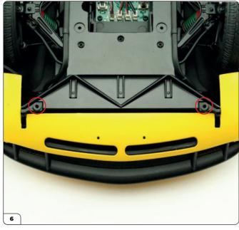
Carefully turn the assembly over then fit the two mounting brackets onto the screw holes in the frame (circled).
