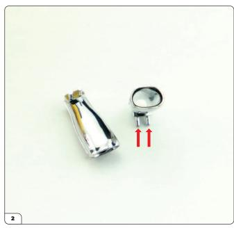
The tailpipes are supplied in bags marked 'R' for right and 'L' for left. They have two silver pins (arrows) for fitting into the holes in the rear body highlighted in step 1.
