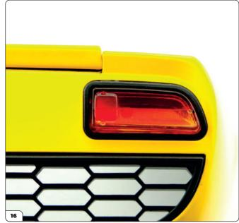
Press the right taillight lens into the housing in the same way.
