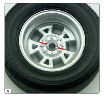
On the inside of the wheel rims are two notches (arrows).
