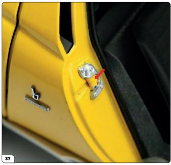
Next you'll install the shims to the door. Open the right side door and locate the space indicated by the arrow.
