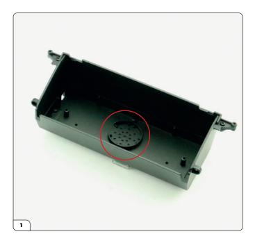
Take the boot compartment assembled in Stage 93 and place it on your work surface as shown. Note there is a circular recess for fitting the speaker (circled).
