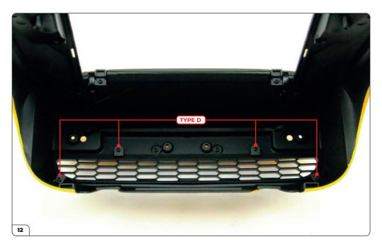
Using 4x Type D screws (supplied with Stage 91) secure the rear grille by driving the screws into the fixing points highlighted in the previous step.
