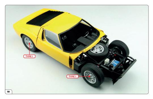
On the other side of the model, fix the last two wheels in place using 2x Type I screws.
