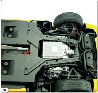
Pull the end of the wire through into the central shaft (arrow).
