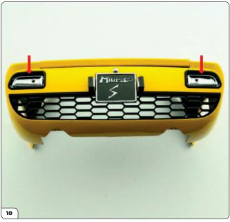
Fit the taillight housings into the corresponding left and right holes in the rear body as shown by the arrows.
