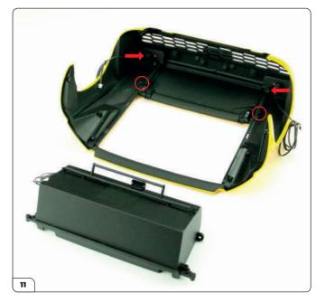
Now you'll install the boot compartent into the rear body. Lay the body upside down as shown on your work surface. Locate the two raised screw holes next to the LED bulbs (arrows) and the two clamp points near the boot lid hinges (circled). Align the compartment with the rear body as shown. Be sure to move the wires of the taillight LEDs aside before fitting the compartment as shown in the image.
