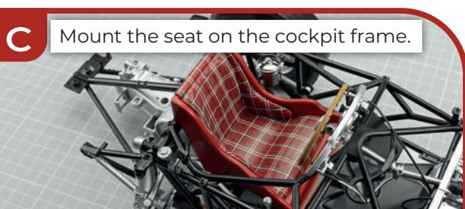
C Mount the seat on the cockpit frame.
