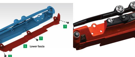
All that remains is to install the lower fascia of the dashboard (5) onto the assembly. Fit the mounting posts into the screw holes as shown and secure by using three type B screws (7).
