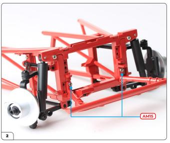
Fit the screw mounts on the subframe base into the corresponding recesses on the assembly and secure in place using 2 x AM15 screws.
