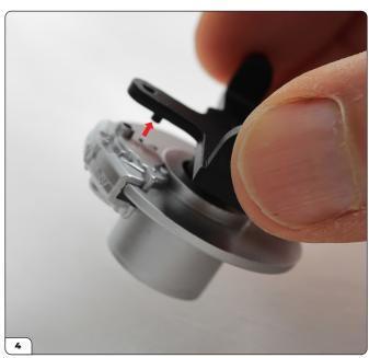
The underside of the caliper fits onto the locating pin.
