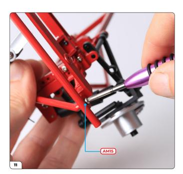
Fix the stay to the front subframe base from the underside using an AM15 screw.
