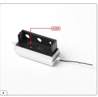
Press the parts firmly together and secure with an AG06 screw.
