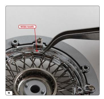
When you fit the first type B spoke, thread it through an empty diamond-shaped opening (see step 12) and check that it will hook around a **wide** tooth on the opposite side as shown here.
