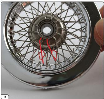
When you thread the type B spoke through to the opposite side, it should cross a type A spoke and fit through an empty diamond-shaped opening. It should lead slightly anti-clockwise. Check that it will hook a wide tooth, but do not hook it just yet, leave the spokes loose.
