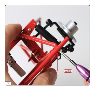
Secure the left stay in place from underneath the subframe using an AM15 screw.
