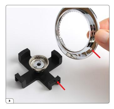
Take the wheel rim and align the hole on the outer edge with the pin on the jig (arrows).
