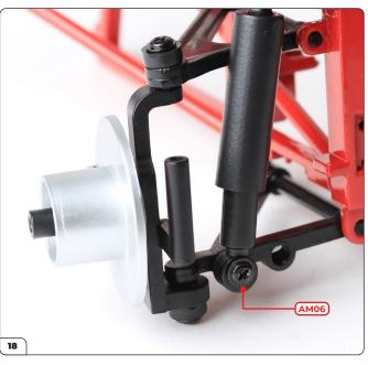
Pushing the spring and the damper body into the shock absorber shroud, fit the eye of the damper body onto the lower wishbone and secure in place with an AM06 screw.
