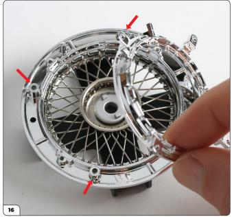
Prepare 4 x AG02 screws and have your screwdriver ready. Carefully align the spoke retainer ring over the wheel. The projecting screw holes on the ring will fit onto the raised screw holes as indicated. Lower the ring into position.
