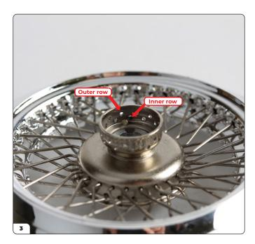
Turn the wheel over so that the smaller side of the wheel centre is facing you. Note that there are two rows for threading the spokes – an inner row and an outer row. You're going to start on the inner row.
