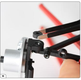
Fit the other suspension bush over the hole and the tip of the lower wishbone.
