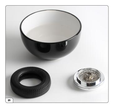
Take the completed wheel and the tyre from stage 15. Prepare a hot water bath by filling a small bowl with boiling water. Soak the tyre in the water for 2 minutes.
