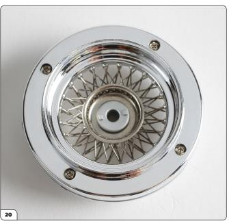
Fix the inner wheel rim in place with 4 x AG03 screws.
