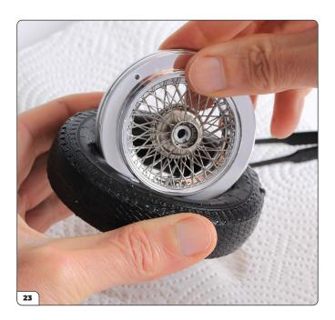
Working quickly while the tyre is pliable, push the wheel into the tyre and twist to fit the outer wheel rim under the inner rim of the tyre.
