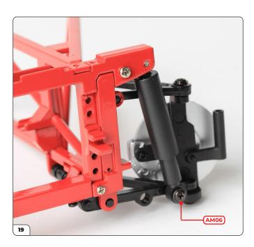
Pushing the spring and the damper body into the shock absorber shroud, fit the eye of the damper body onto the lower wishbone and secure in place with an AM06 screw.
