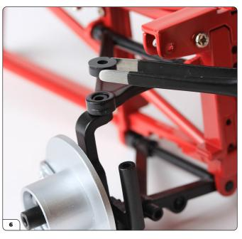
Fit the ends of the upper and lower wishbones onto the suspension upright. Fit a suspension bush over the hole on the upper wishbone.
