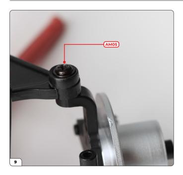
Secure the suspension bush to the suspension upright with an AM05 screw. Do not overtighten the screw as the upright must be free to
