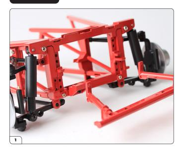
Align the front subframe base with the bottom of the assembly from stage  $28.\,$
