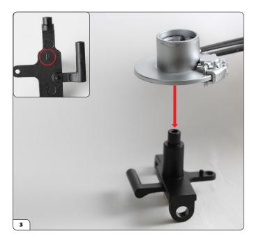
Fit the brake disc onto the central part of the left suspension upright, ensuring that the caliper is aligned with the locating pin. Note: if the suspension upright supplied is marked with an 'R', check Stage 28 to find the left suspension upright, marked 'L'.
