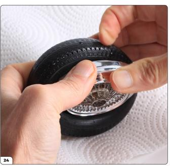
Keep pushing and pulling, working around the tyre, until the side walls fit comfortably over the wheel rim on both sides.
