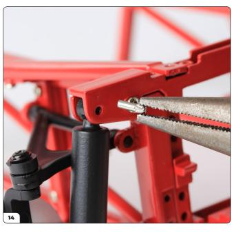
Using pliers, push the smooth end of the pivot pin into the hole on the subframe, making sure it goes through the eye of the shock absorber shroud.
