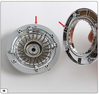
Take the inner wheel rim and align the four screw holes and the pin (arrowed). Prepare  $4 \times AGO3$  screws and a screwdriver.
