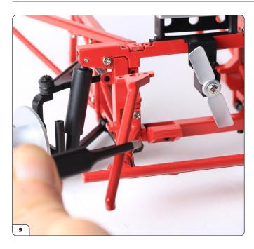
Repeat steps 6, 7 and 8 to fix the front subframe right stay in place on the opposite side: start by aligning the stay...
