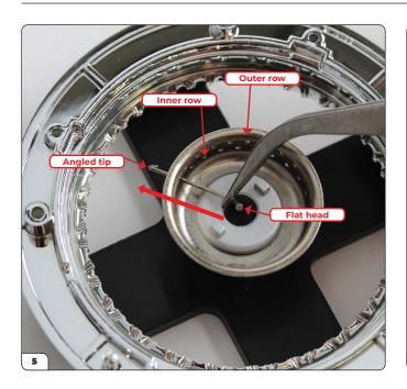
Before you begin, note that the inner edge of the spoke retainer ring has a series of 'teeth', alternating in size (see picture 6). Each spoke has a right-angled tip, and a flat head on the opposite end. Use your tweezers to thread the spokes and hook them into place. Start by threading a spoke, leading with the tip, through a hole in the innermost row of holes in the wheel centre.
