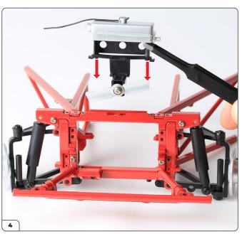
Lower the cooling fan assembly from stage 30 onto the subframe (see step 5).
