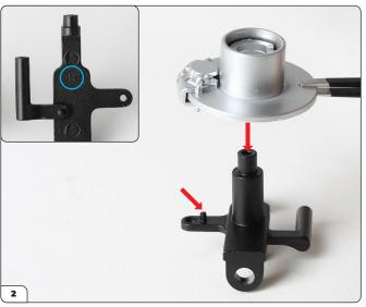
Fit the brake disc onto the central part of the right suspension upright, ensuring that the caliper is aligned with the locating pin.
