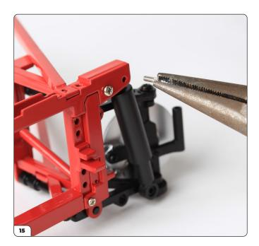
Take the pivot pin and note that one end is smooth, the other end is splined. Using pliers, push the smooth end of the pin into the hole on the subframe, making sure it goes through the eye of the shock absorber shroud.
