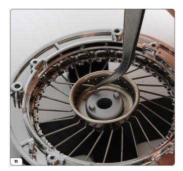
Start in the same way, threading the tip of a spoke through a hole in the uppermost row.
