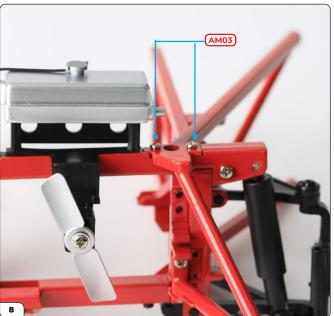
Use another 2 x AM03 screws to fix the stay to the top of the subframe.
