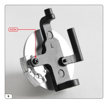
Secure the caliper to the upright with an AG04 screw.
