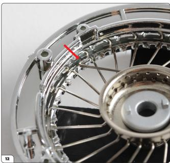
The spoke tips will now face in the opposite direction to those fitted on the bottom row. Make sure that they are hooked around a 'wide' tooth otherwise they cannot be secured in place in a later step.
