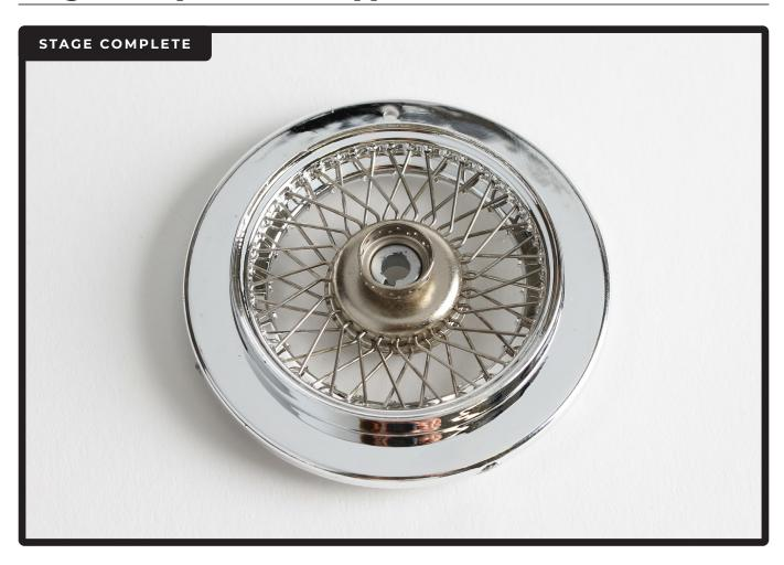
In this next stage you will complete the wheel, lacing more spokes and fitting the tyre.
