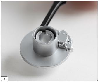
Slot the caliper onto the brake disc.
