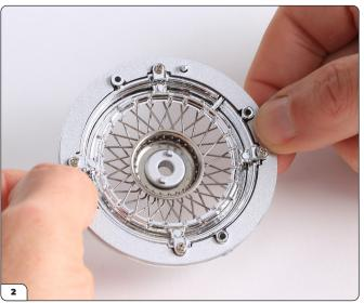
Lower the ring onto the wheel and press firmly until it clicks into place.
