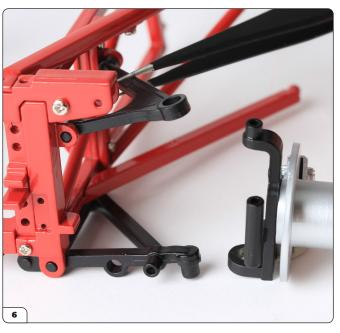
Align the brake disc assembly with the upper and lower wishbones on the subframe from stage 26.
