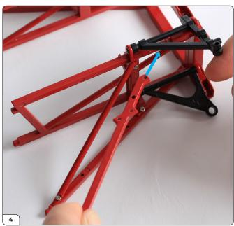
With the subframe assembly upside down on your worksurface, take the left-hand lower brace and feed it between the lower wishbone and the bottom of the subframe (see also step 5).
