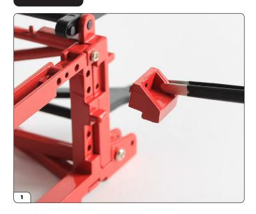
Align the steering rack mounting bracket with the front crossmember on the subframe assembly from stage 22.
