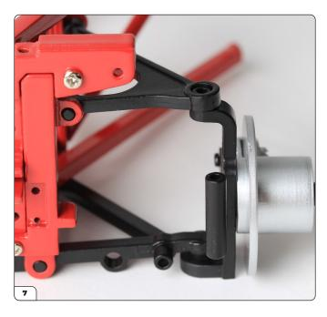
Fit the ends of the wishbones onto the suspension upright.
