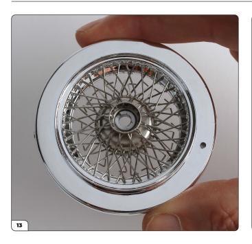
All 12 x type B spokes have been fitted to the outer row of the wheel centre and are left loose on the underside.
