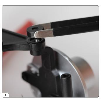
Fit a suspension bush over the hole on the upper wishbone.
