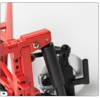
The pivot pin is now securing the shock absorber shroud in place.
