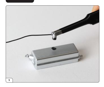
Align the filler cap with the header tank.
