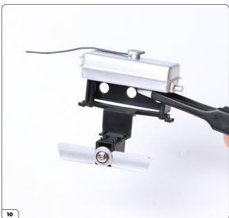
Press the parts firmly together and secure them in place using 2  $\times$  AG04 screws.
