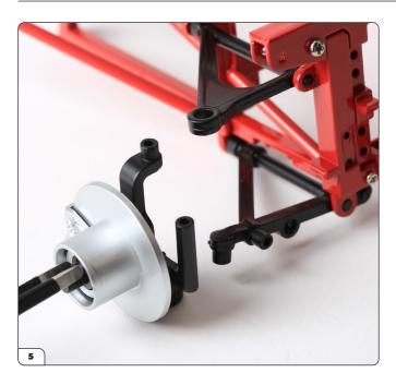
Align the brake disc assembly with the upper and lower wishbones on the subframe.
