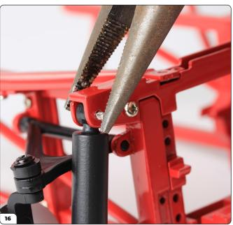
Squeeze the pin with pliers to press it fully into the hole.
