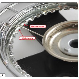
Pull the spoke through the hole and hook the tip around the nearest 'wide' tooth that gives the spoke a comfortable fit.
