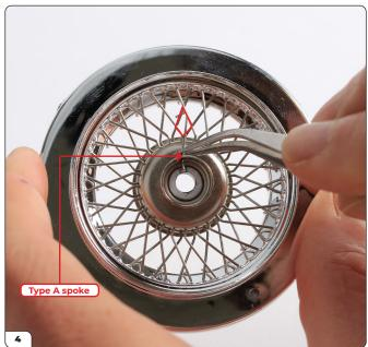
Using tweezers, thread a type A spoke through a hole on the **inner row**. Direct the tip of the spoke through the diamond-shaped opening slightly clockwise (coloured red above) so that the tip pokes through to the opposite side.
