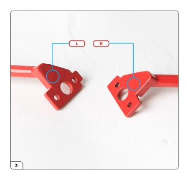
Before preparing to fit the cooling fan, take the front subframe stays and note that they are marked left (L) and right (R).
