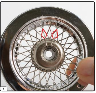
Once you are happy that the first spoke is fitted correctly, thread the next spoke through an adjacent hole in the lower row, but this time, poke it through the diamond-shaped hole that is two-along.
