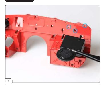
Align the three pins on the heater case with the three holes on the bulkhead (circled).
