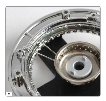
Then take another spoke and thread it through the next hole in the innermost row of the wheel centre. Pull the spoke through the hole and hook the tip around the next 'wide' tooth.
