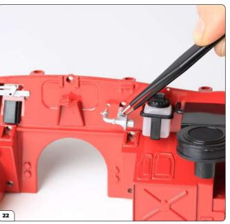
Line up the heater water control valve next to the reservoir.
