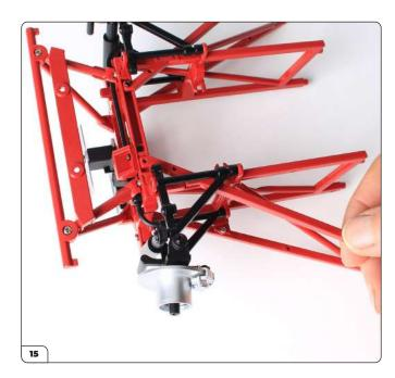
Take the right-hand lower brace from stage 26 and fit it across the subframe with the screwhole in the end aligned with the second screwhole on the steering rack mounting.
