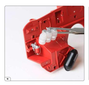
Align the fluid reservoirs with the mounting holes on the bulkhead.
