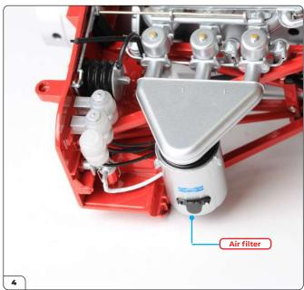
Before fixing anything, check that the bunch of black pipes are not trapped under the frame and that they are free to be moved behind the air filter. See step 16 for more guidance.
