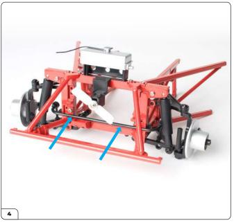
Position the anti-roll bar on the front of the subframe, within the triangles formed by the diagonal stays at the front of the subframe.
