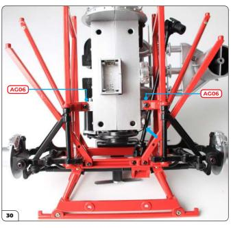
Carefully slide the engine into place so that the engine mounts line up with the mounting points on the underside of the subframe. Secure the engine mounts on both sides using  $2 \times AG06$  screws. Note the angle of the steering column (arrow).
