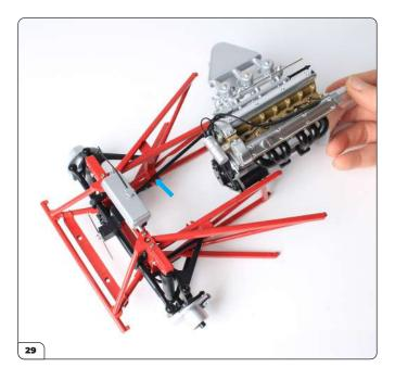
Now it's time to fit the engine to the subframe. Start by lining up the engine within the rear of the subframe. Make sure the steering column is kept to the side and out of the way, resting on the mounting point indicated.
