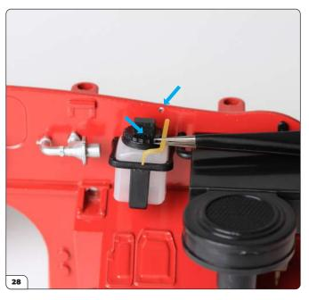
Fit one end of the washer tube into washer reservoir cap and the other end into the bulkhead as shown (see step 29).
