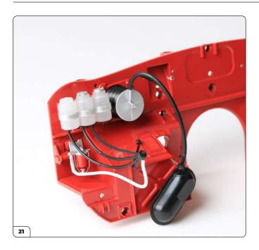
A brake vacuum hose has been connected to the brake servo, leaving one brake vacuum hose to be connected at a future stage.
