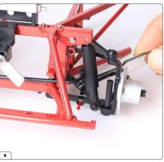
Feed the pins on the end of the links into the holes in the bottom wishbone.
