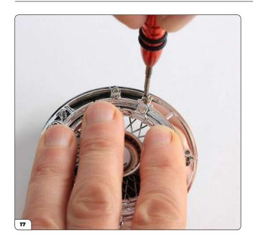
Hold the retainer in position so that the spokes are secured as you fit an AG02 screw.
