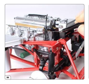
Locate the end of the hose leading from the filler cap on the expansion tank...
