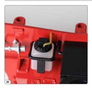
The washer tube is fitted into place.
