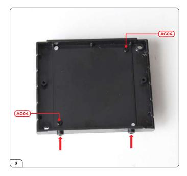
Turn the radiator/cowl assembly over so the reverse side is facing you and note that there are two lugs along one edge (arrows). Secure the cowl to the radiator with  $2 \times AGO4$  screws.
