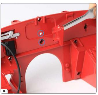
Align the two pins on the engine stabiliser mounting with the two holes on the bulkhead (circled).
