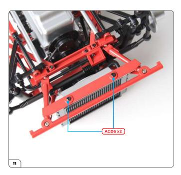
Secure the radiator in place from the underside using 2 x AG06 screws.
