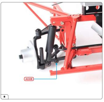
Fit the link on the other end of the anti-roll bar in the same way, securing it with another AG08 screw.
