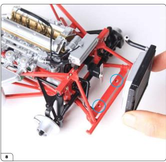
Align the two lugs on the bottom of the radiator (see step 3) with the two holes in the bottom bar of the front subframe (circled).
