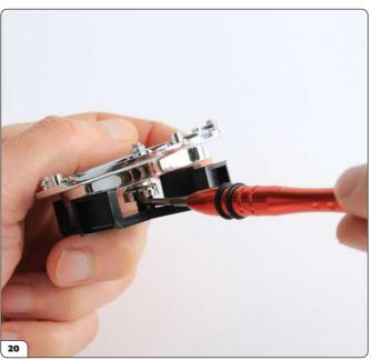
Gently prise the wheel off the jig. Do not pull the wheel – try to carefully release it using a screwdriver or similar tool that will act as a lever.
