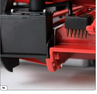
Position the assembly on the subframe, just below the heater motor.
