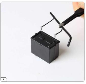
Next, you'll install the battery. Start by plugging the battery leads into the battery by positioning them as shown.
