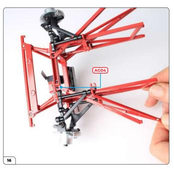
Secure the right-hand lower brace to the steering rack mounting using an AG04 screw. Be careful not to over tighten this screw.
