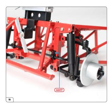
Repeat the process on the opposite end of the anti-roll bar, securing the second mounting in place with another AM17 screw.
