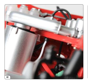
Push the pin firmly into the subframe.
