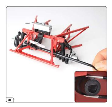
Now feed the steering rack assembly through the triangular braces at the front of the subframe. Check that the teeth on the rack are positioned so that they will align with the gear.
