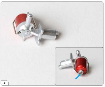
Check that the middle section of the clip fits on the fuel filter as shown (inset arrow). If necessary, secure the clip with a tiny drop of superglue.
