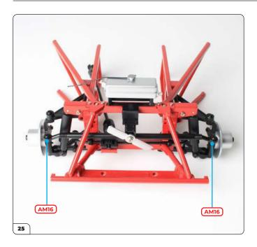
Secure the steering rack to each upright using an AM16 screw
