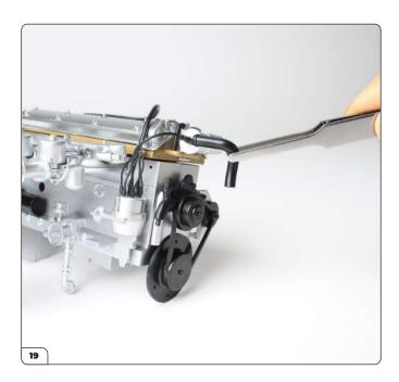
Fit the water hose by pushing one end over the pin on the water pump, and tuck the other end behind the plug leads.
