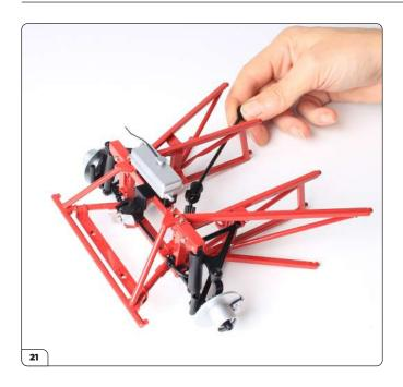
Returning to the subframe assembly, feed the steering column assembly through the subframe until the gear at the end of the steering column sits in the steering rack mounting (see step 22).
