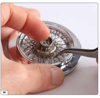
Fit the type B spokes to the outer row of the wheel centre, just above the type A spokes.
