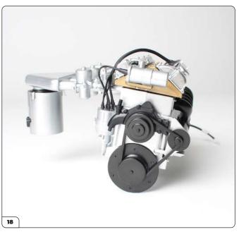
Fit the water pump behind the uppermost pulley.
