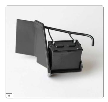
Push the lug on the bottom of the battery into the hole in the mudshield.
