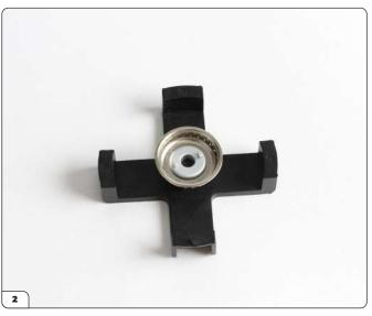
Fit the wheel centre onto the jig.
