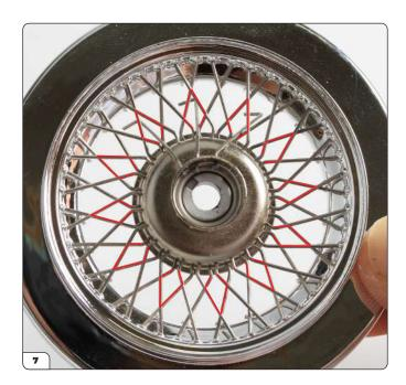
Continue to thread the type A spokes all the way around the inner row, pushing the tip through alternate diamond-shaped openings as indicated.
