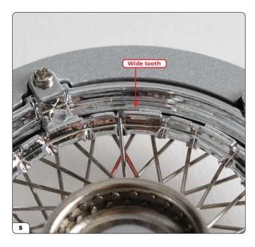
Turn the wheel over and check that the tip will hook onto a wide tooth on the opposite side. If it doesn't fit a wide tooth, start again, threading the spoke through the next diamond-shaped hole along.
