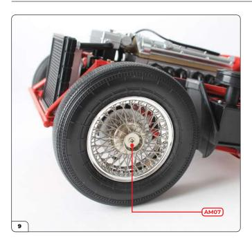
Secure the washer and left wheel in place using a type AM07 screw.
