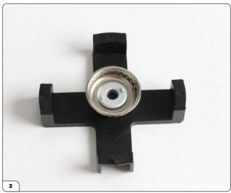
Fit the wheel centre onto the jig.
