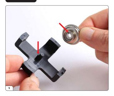
Take the wheel centre and note that there is a small notch that aligns with a corresponding tab on the jig (arrows). The jig is used here to assist with building the wheel and will be removed towards the end of the wheel-build.
