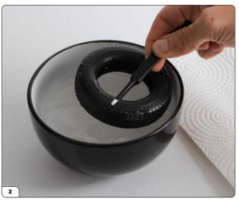
Carefully remove the tyre from the water bath using tongs or tweezers - the tyre will be very hot! Shake off any excess water and dab on kitchen paper or a towel.
