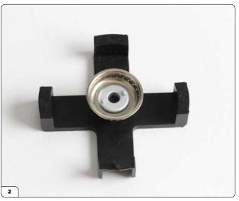
Fit the wheel centre onto the jig.
