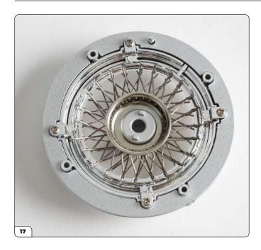
Spokes A and B are correctly hooked in place around the teeth.
