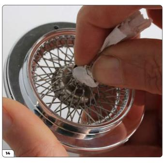
Use a piece of cotton wool or kitchen paper to hold the pin ends of the spokes in place in the inner and outer rows of the wheel centre.
