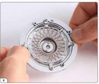
Lower the ring onto the wheel and press firmly until it clicks into place.
