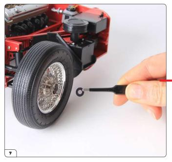
Take the washer and place it into the end of the stub axle, as shown in picture  $8. \,$
