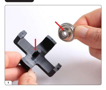
Take the wheel centre and note that there is a small notch that aligns with a corresponding tab on the jig (arrows). The jig is used here to assist with building the wheel and will be removed towards the end of the wheel-build.
