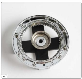
Fit the wheel rim onto the jig, pressing firmly to lock the rim into position.  $\;$
