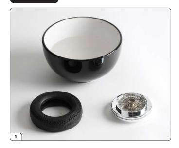
Take the completed wheel from Stage 52. Prepare a hot water bath by filling a small bowl with boiling water. Soak the tyre in the water for 2 minutes.
