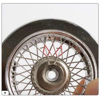
Once you are happy that the first spoke is fitted correctly, thread the next spoke through an adjacent hole in the lower row, but this time, poke it through the diamond-shaped hole that is two-along.
