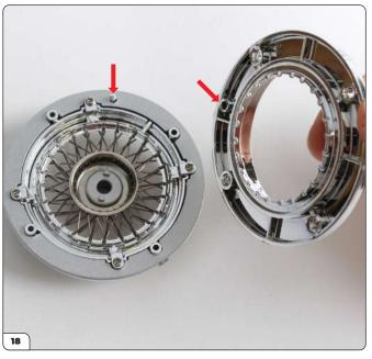
Take the inner wheel rim and align the four screw holes, and the pin with its corresponding hole (arrows). Prepare  $4\times AG03$  screws and a screwdriver.
