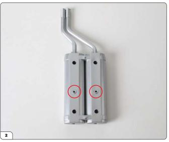
Place the upper half onto the lower half of the silencer, so that the long posts fit through the holes (circled).
